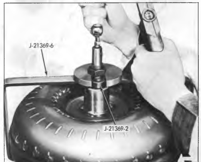
Figure 105—Air Checking Converter
