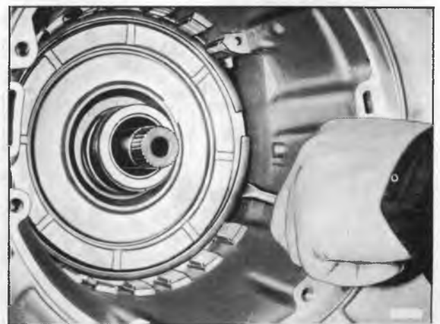
Figure 31—Removing Center Support to Case Snap Ring
