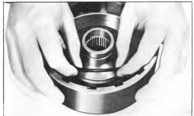
Figure 79—Installing Direct Clutch Center Seal
