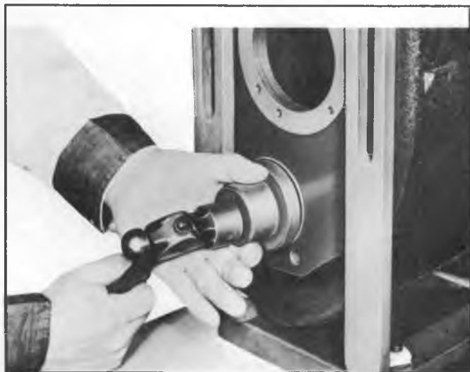
Fig. 26R-Installing Countershaft Front Bearing Spacer
