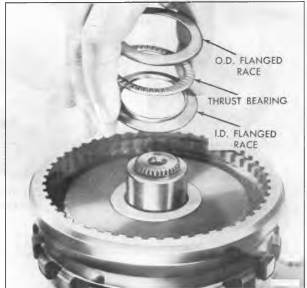
Figure 109—Installing Rear Internal Gear to Output Shaft Bearing and Races
