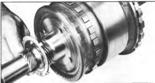
Figure 118—Installing Case to Output Shaft Thrust Washer
