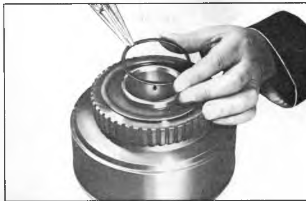
Figure 86—Installing Retainer Snap Ring
