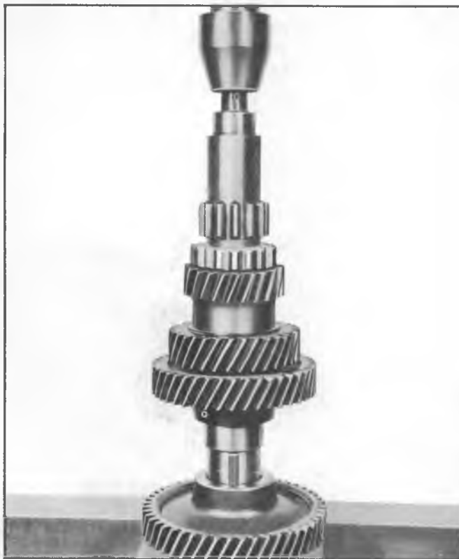
Fig. 22R--Installing Countershaft Drive Gear
