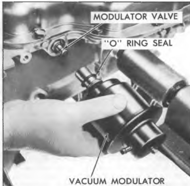
Figure 4—Removing Vacuum Modulator and Valve
