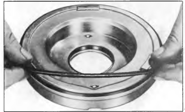
Figure 78—Installing Direct Clutch Outer Seal
