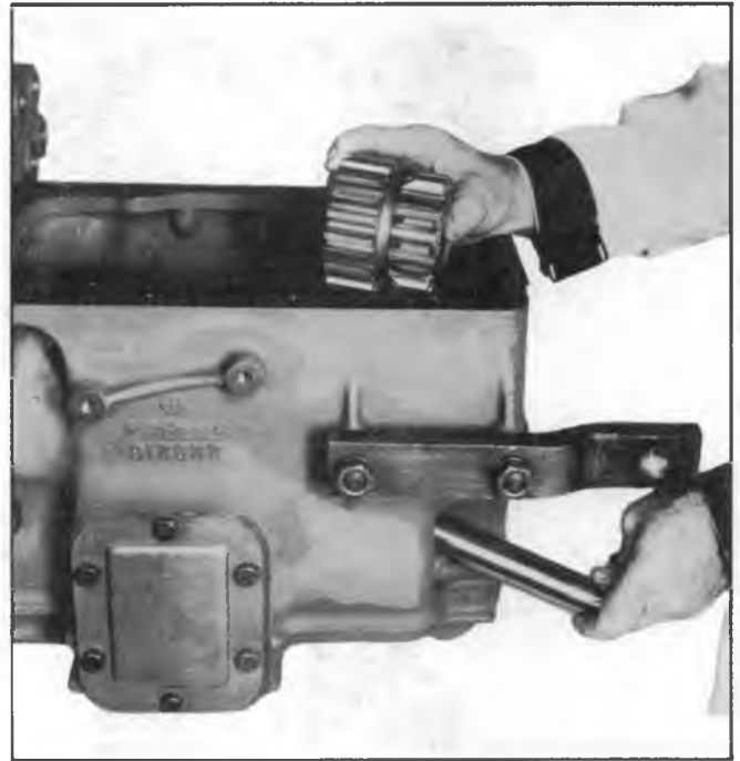
Fig. 10N--Removing Idler Gear and Bearings
