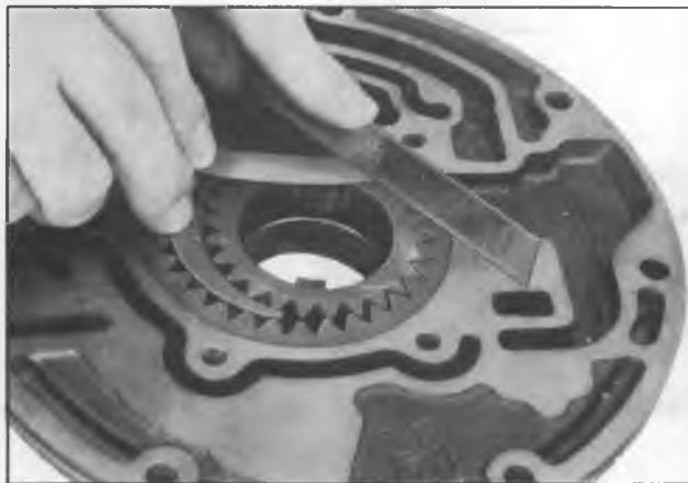
Figure 58—Checking Pump Body Face to Gear Face Clearance
