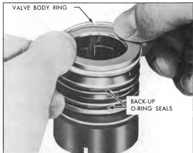
Fig. 27--Installing Valve Body Rings
