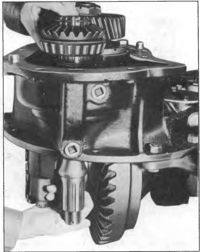
Fig. 25M—Installing Output Shaft Assembly
