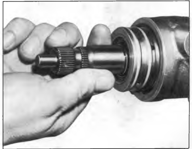
Fig. 19--Removing Valve Assembly
