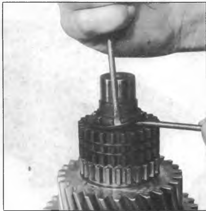
Fig. 13N--Removing 4th and 5th Shift Hub Sleeve Retainer Ring
