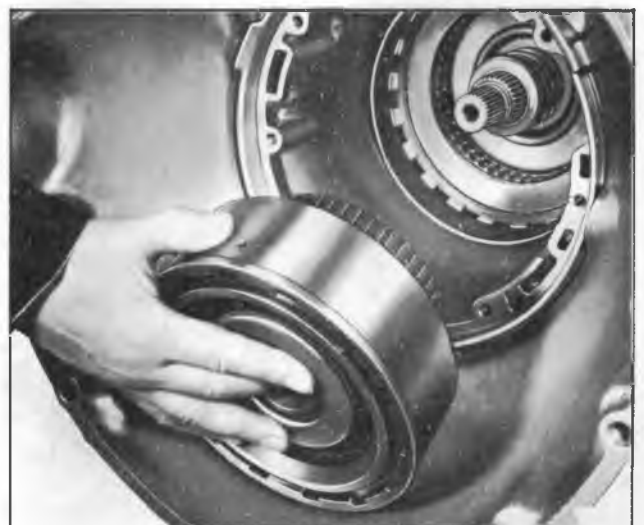
Figure 24—Removing Direct Clutch Assembly
