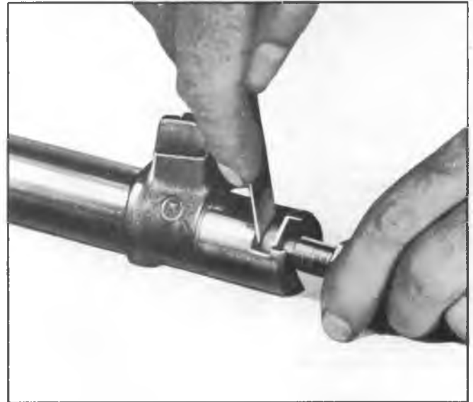
Fig. 9--Checking Lash Adjuster End Clearance
