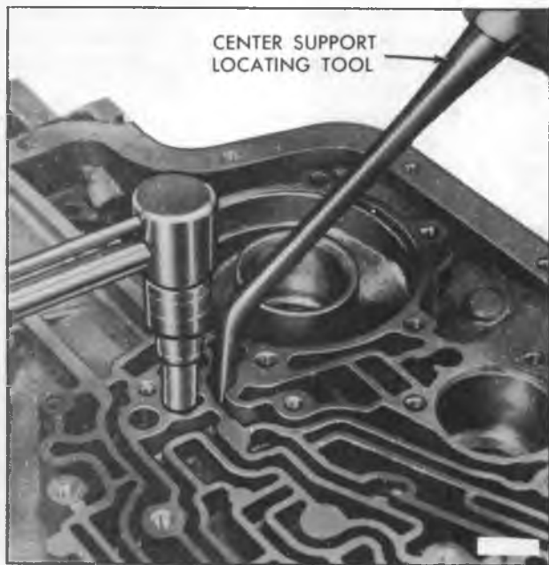
Figure 122—Installing Case to Center Support Bolt
