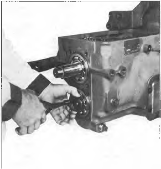
Fig. 6N--Removing Countershaft Rear Bearing Retainer Ring
