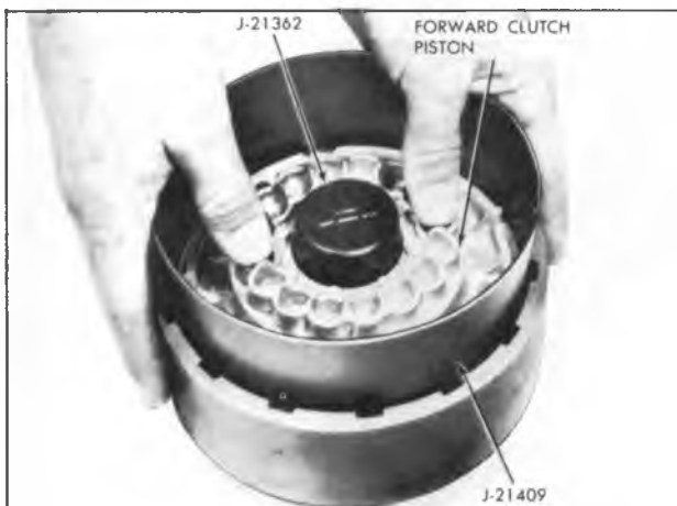
Figure 69—Installing Forward Clutch Piston
