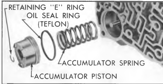
Figure 51—Removing Front Accumulator Piston and Spring
