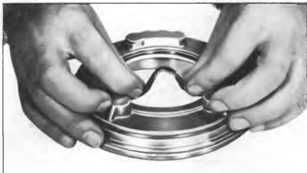
Figure 91—Installing Intermediate Clutch Inner Seal
