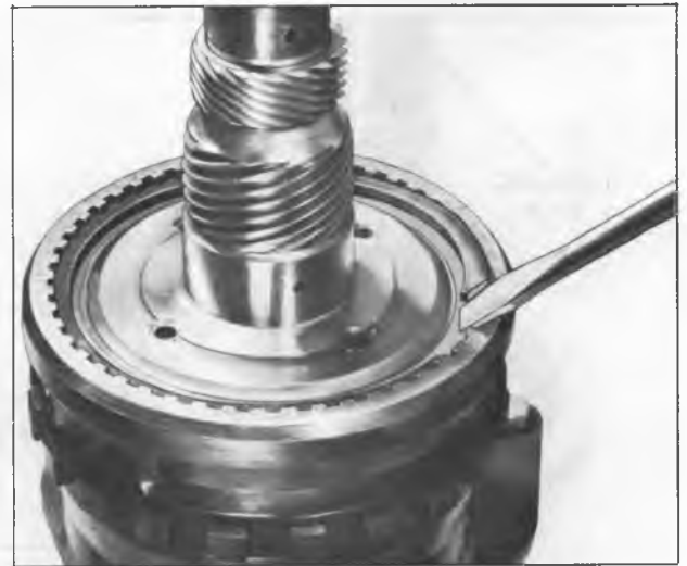
Figure 38—Removing Output Shaft to Carrier Snap Ring
