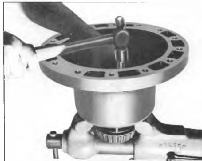
Fig. 21J--Removing Differential Bearings Using Brass Drift
