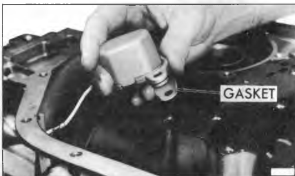
Figure 15—Removing Detent Solenoid and Gasket
