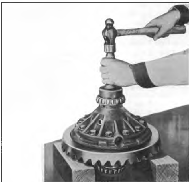
Fig. 14G--Differential Bearing Installation
