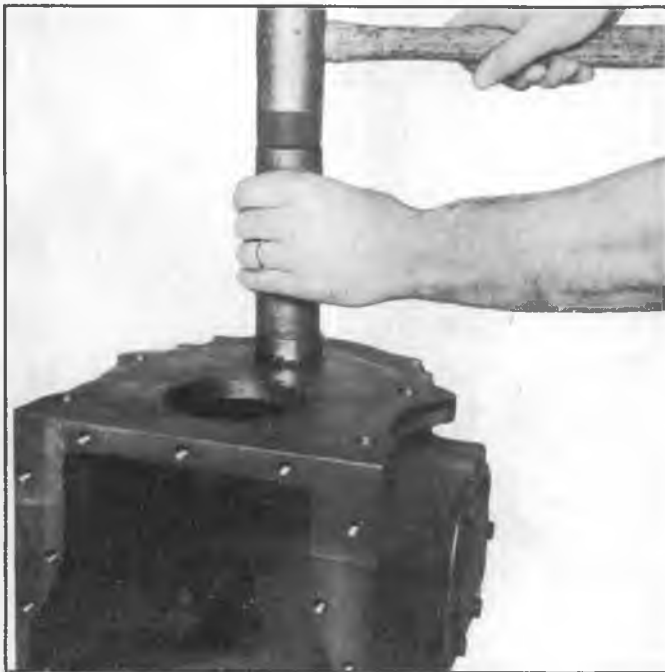
Fig. 21N--Installing Countershaft Front Bearing
