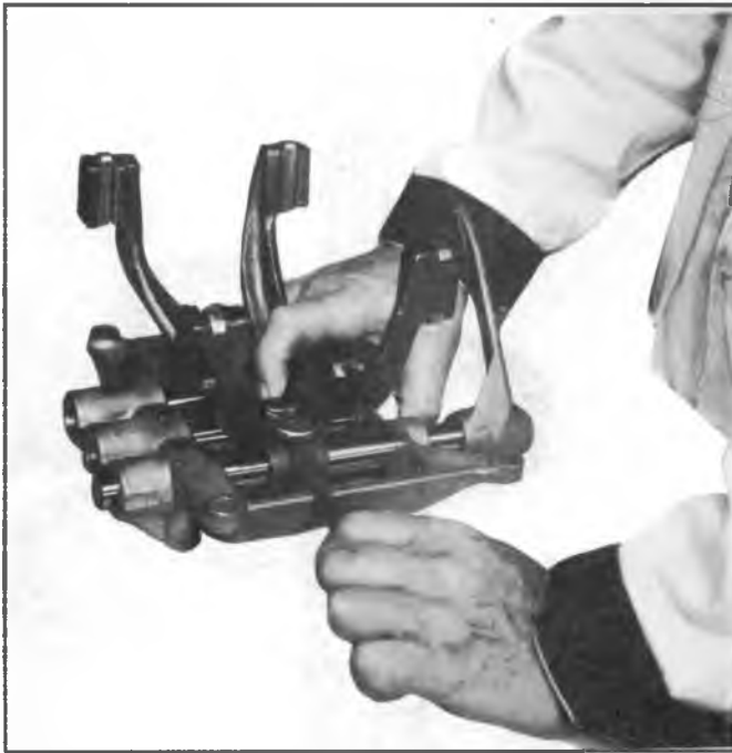
Fig. 16N--Removing 1st and Reverse Shift Lug Lockscrew
