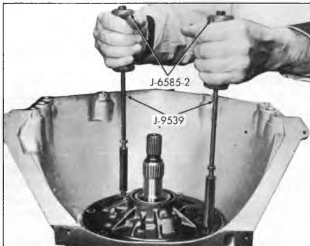
Figure 22—Removing Pump Assembly
