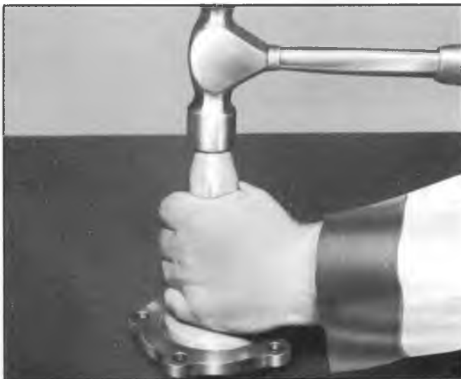
Fig. 8G--Pinion Oil Seal Installation (Typical)
