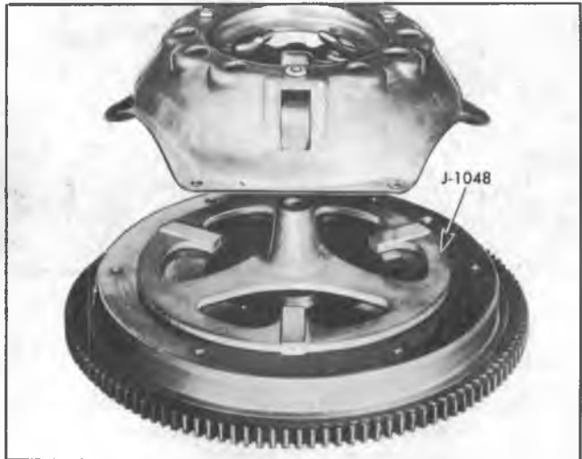
Fig. 12E--Gauge Plate Position (Typical)
