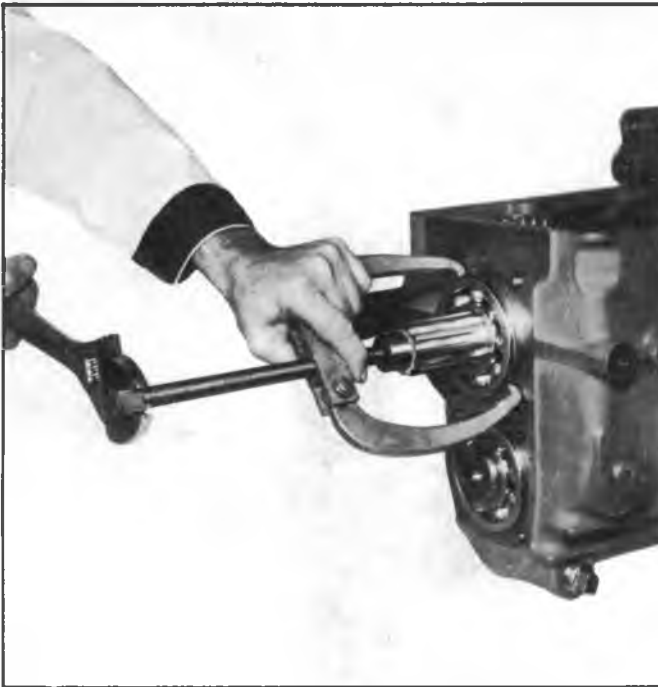
Fig. 8N--Removing Mainshaft Rear Bearing
