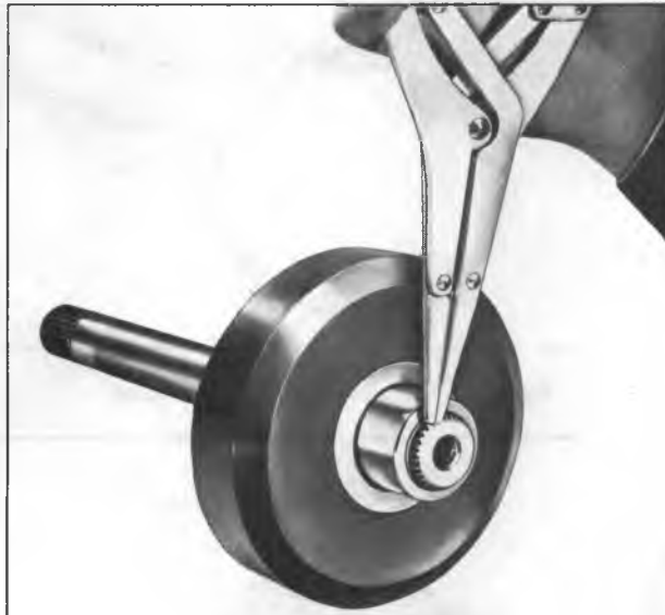
Figure 107—Installing Rear Internal Gear Snap Ring
