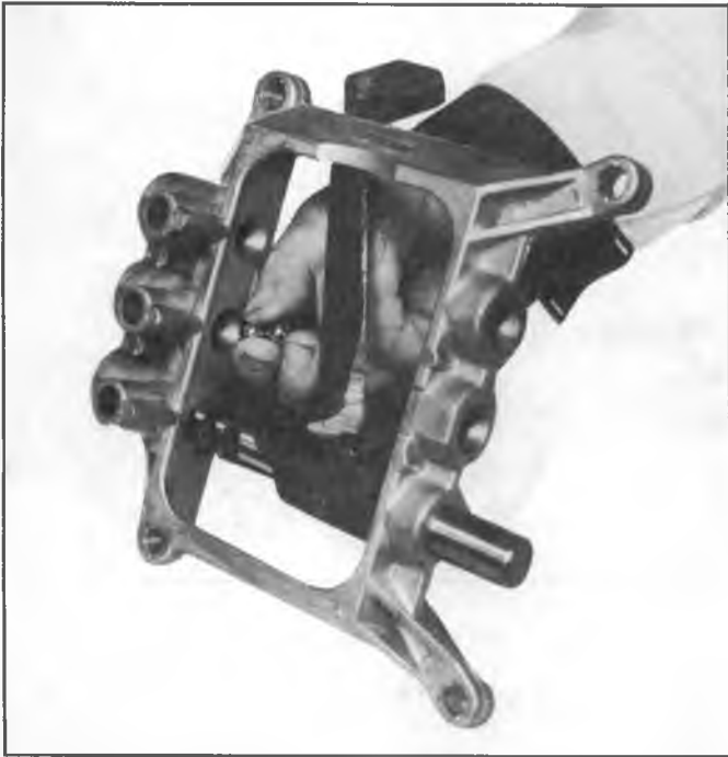
Fig. 20N--Installing Interlock Balls
