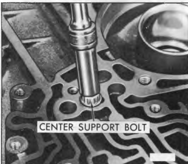
Figure 29—Removing Center Support to Case Bolt
