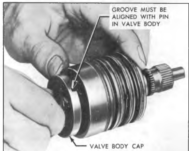
Fig. 25--Removing Valve Spool
