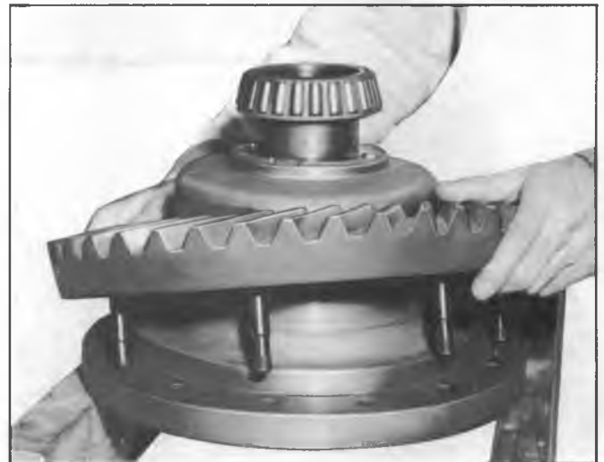
Fig. 23J--Installing Ring Gear Using Improved Guide Pins
