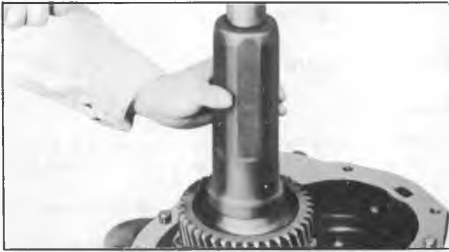
Fig. 23M—Installing Pinion Shaft Helical Gear
