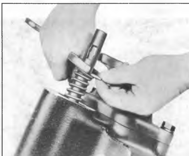
Fig. 8M--Removing Shift Spring, Fork and Clutch
