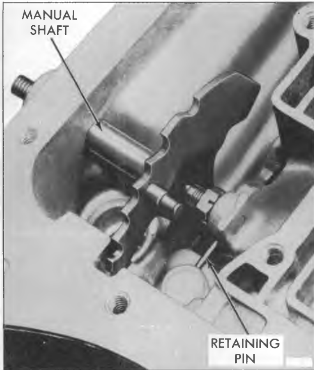
Figure 25—Removing Manual Shaft Retaining Pin
