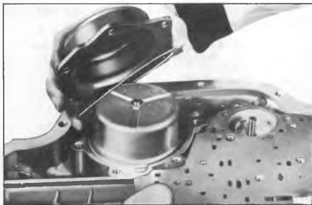
Figure 133—Installing Rear Servo Cover and Gasket
