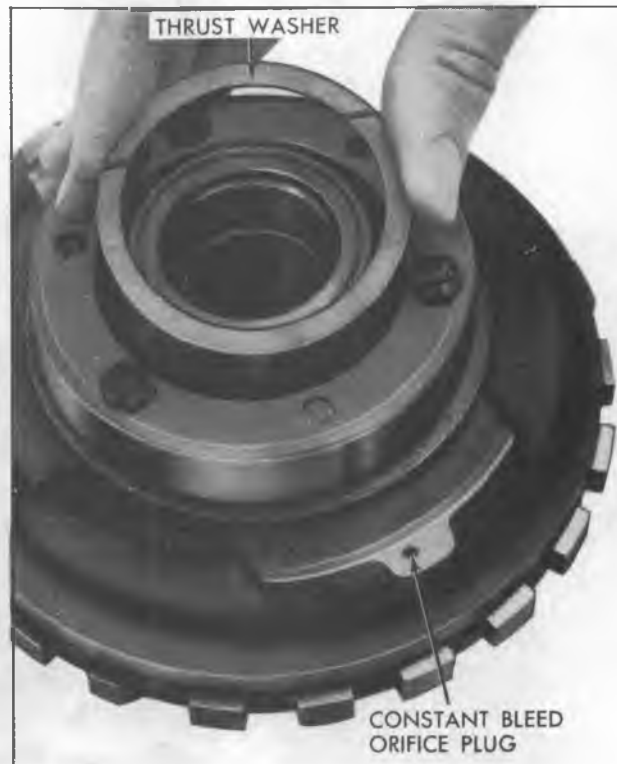
Figure 35—Removing Center Support Thrust Washer
