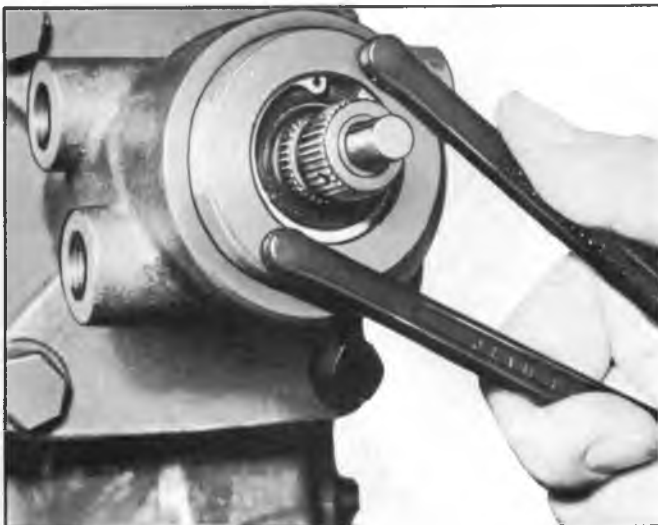
Fig. 18--Removing Adjuster Plug Assembly Using Tool J-7624
