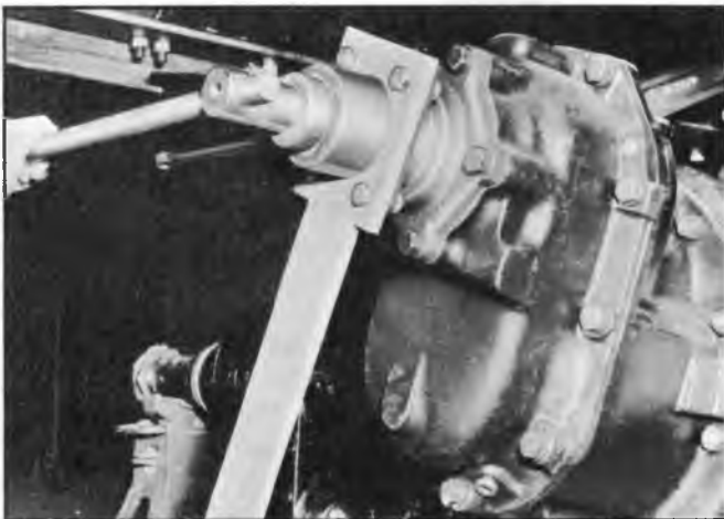
Fig. 3M—Removing Input Shaft Flange Nut
