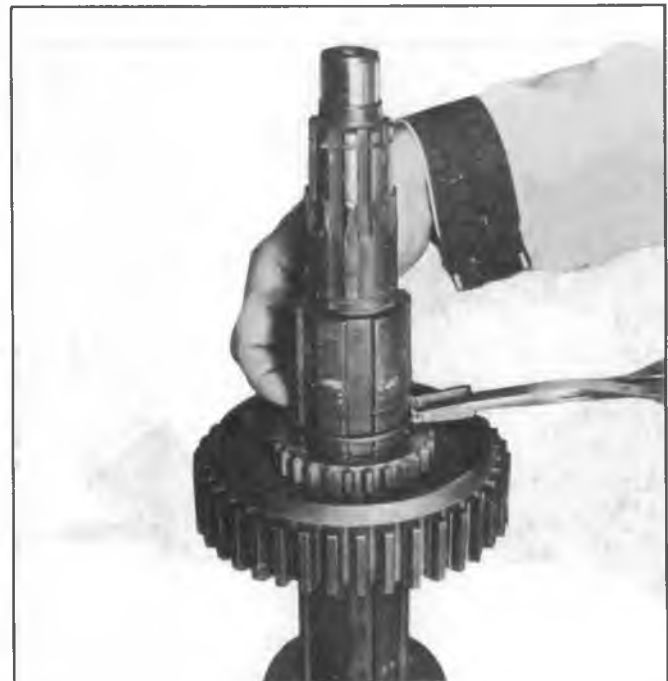
Fig. 15N--Removing 2nd Gear Retainer Ring
