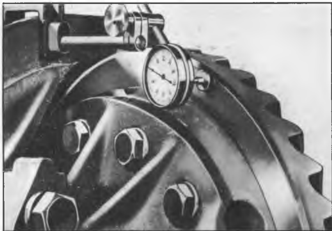
Fig. 6K--Checking Ring Gear Run Out
