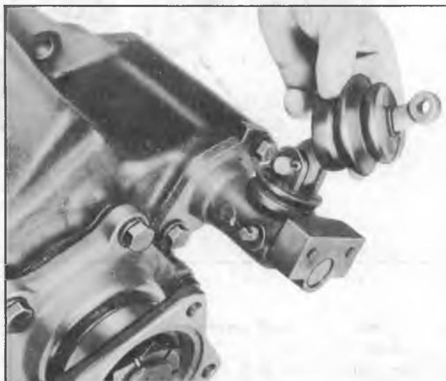
Fig. 7M--Removing Inter-Axle Lock Out Shift Lever
