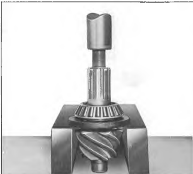
Fig. 10J--Removing Pinion Intermediate Bearing Using J-6203
