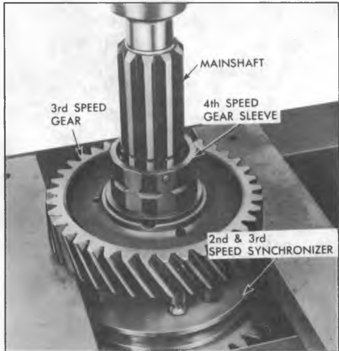
Fig. 16R--Removing Mainshaft from 3rd Gear
