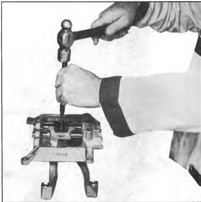
Fig. 17N--Removing 2nd and 3rd Shift Fork Roll Pin
