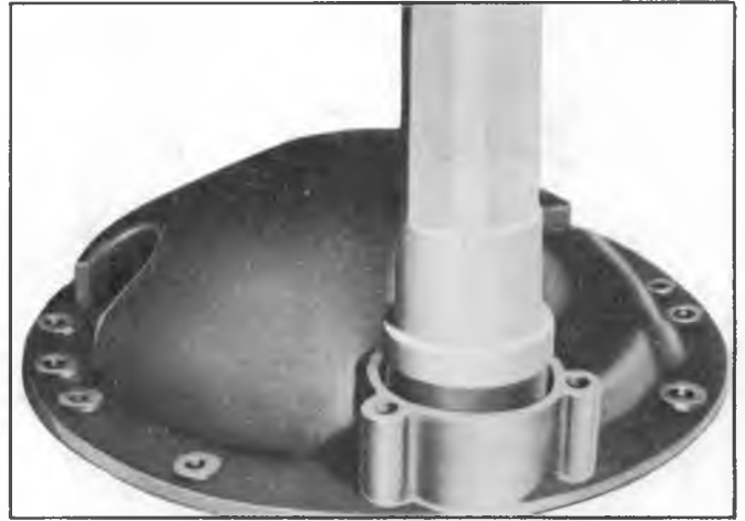
Fig. 28M--Installing Output Shaft Bearing in Cover Using Tool J-6419-1 and -4
