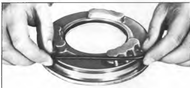
Figure 92—Installing Intermediate Clutch Outer Seal
