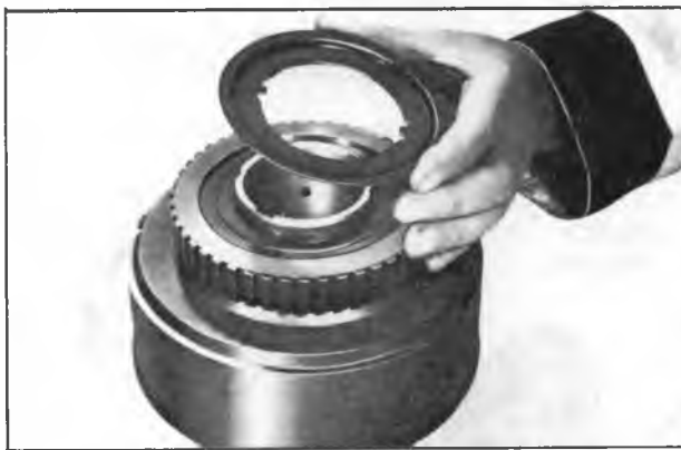
Figure 85—Installing Intermediate Clutch Retainer
