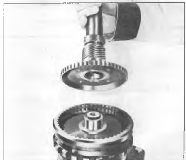
Figure 110—Installing Output Shaft
