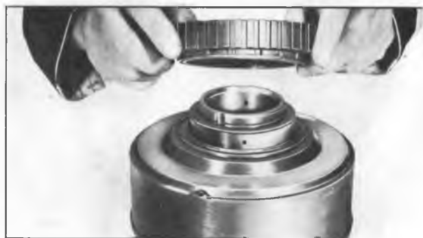
Figure 83—Installing Intermediate Sprag to Direct Clutch
