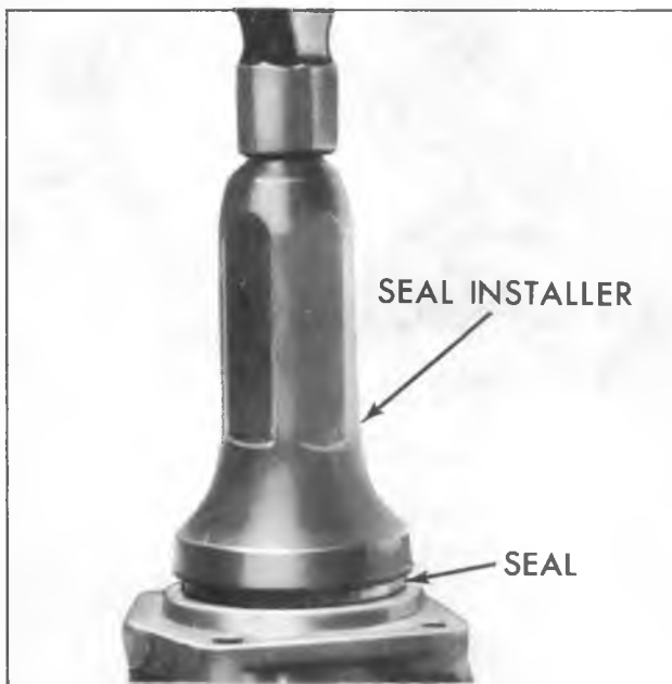
Figure 126—Installing Rear Extension Seal (Using Tool J24057)
