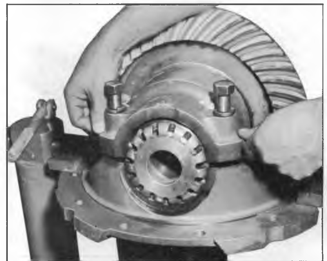
Fig. 24J--Installing Differential Bearing Caps
