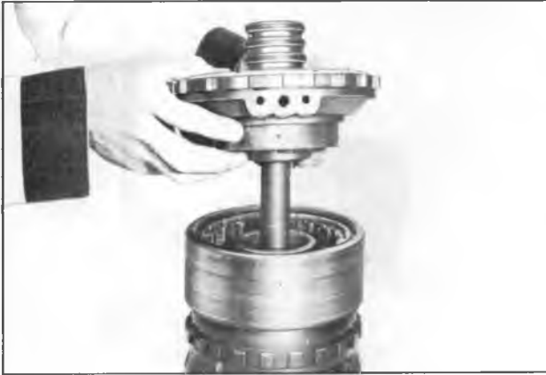
Figure 117—Installing Center Support into Reaction Carrier and Roller Clutch Assembly
