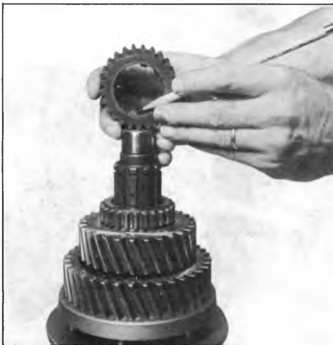
Fig. 24N--Installing 4th and 5th Shift Hub Sleeve
