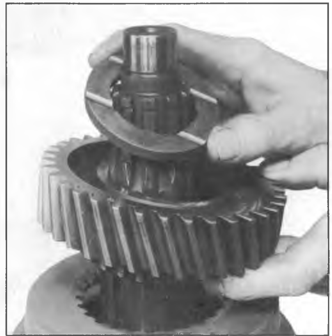
Fig. 23N--Installing 3rd Speed Gear and Washer
