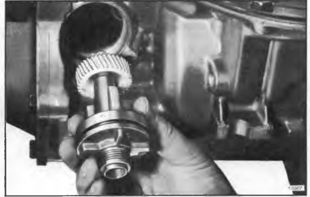
Figure 138—Installing Speedometer Driven Gear
