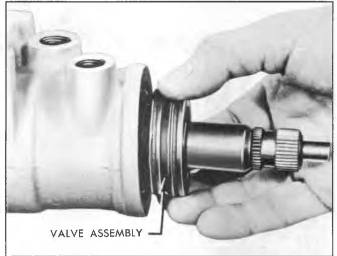
Fig. 33--Inserting Valve into Housing
