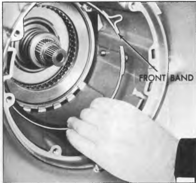
Figure 27—Removing Front Band
