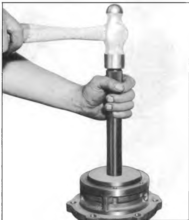
Fig. 14J--Installing Pinion Intermediate Bearing Outer Race
