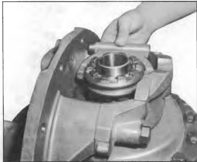
Fig. 5J--Removing Shifter Yoke and Sleeve
