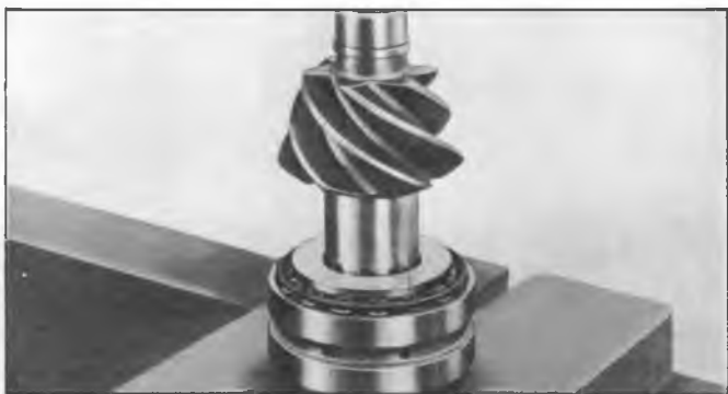
Fig. 11G--Pinion Front Bearing Installation (13,500, 15,000 and 17,000 Lb. Axles)
