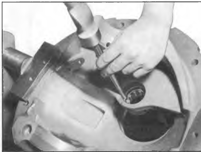
Fig. 13J--Removing Pinion Rear Bearing from Carrier
