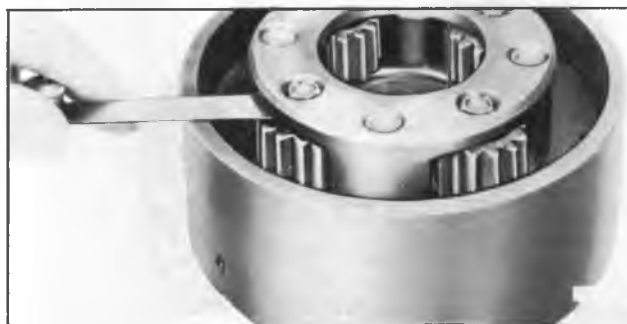
Figure 95—Checking Pinion End Play
