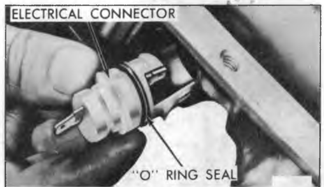
Figure 16—Removing Electrical Connector and O-Ring
