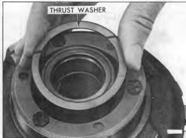
Figure 116—Installing Center Support to Reaction Carrier Thrust Washer
