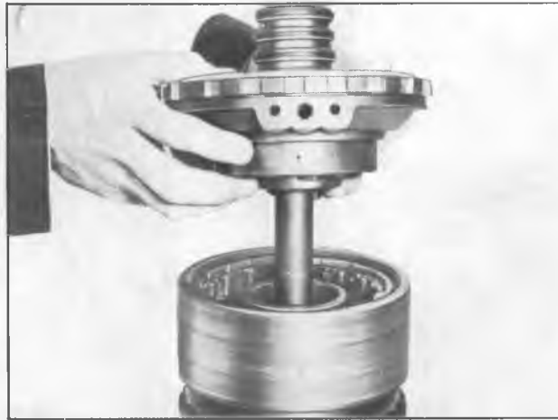
Figure 34—Removing Case Center Support Assembly
