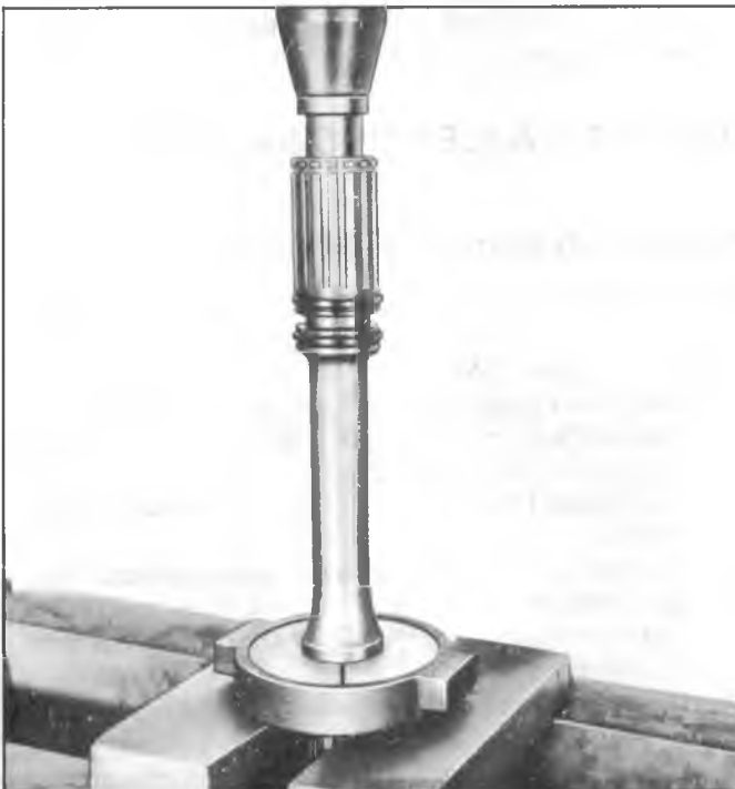
Fig. 21M--Installing Output Shaft Bushing Using Tool J-8476
