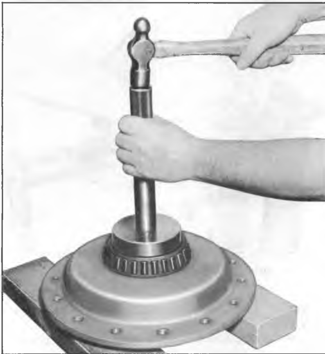
Fig. 22J--Installing Differential Bearings
