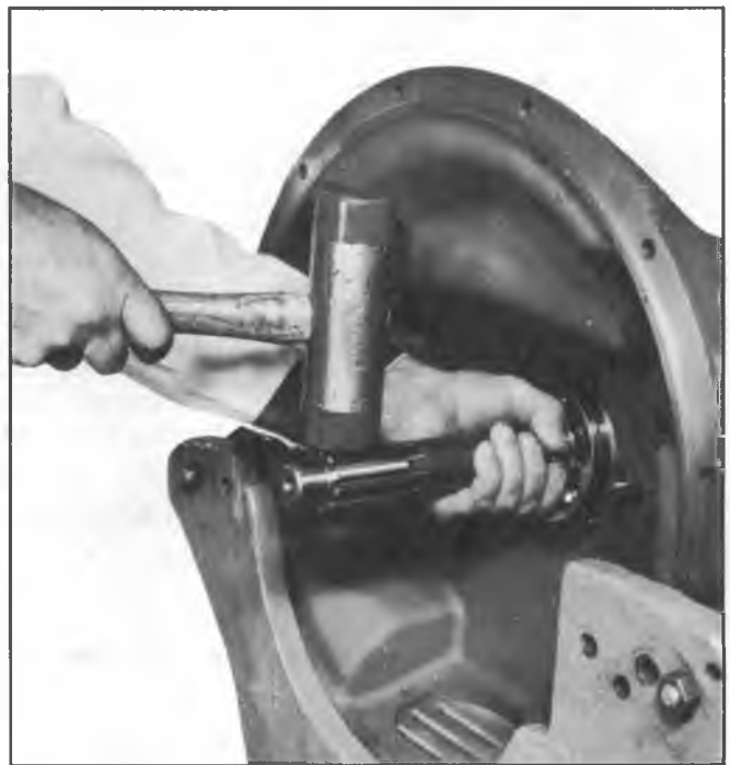
Fig. 7N--Removing Main Drive Gear
