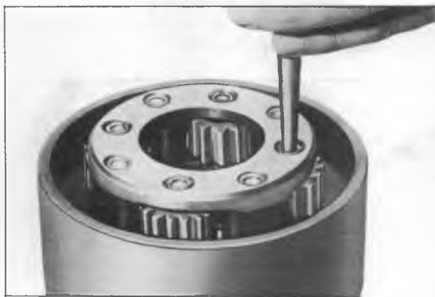
Figure 97—Removing Planet Pinion Pin
