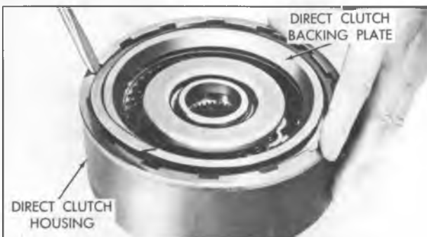
Figure 73—Removing Direct Clutch Backing Plate Snap Ring
