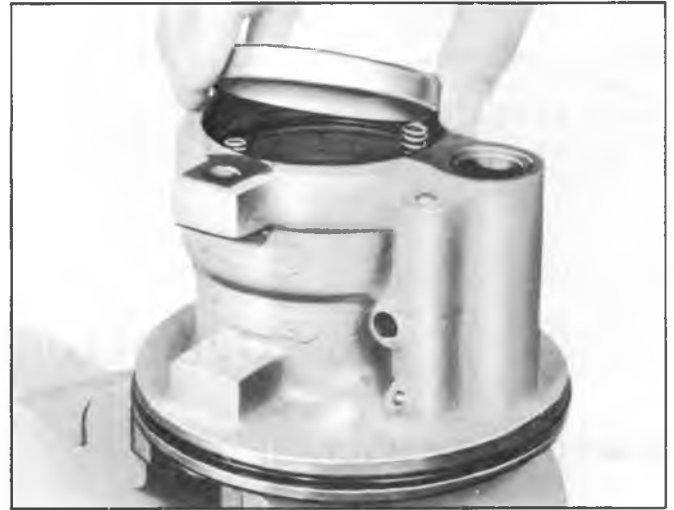
Fig. 16--Installing Pressure Plate Springs
