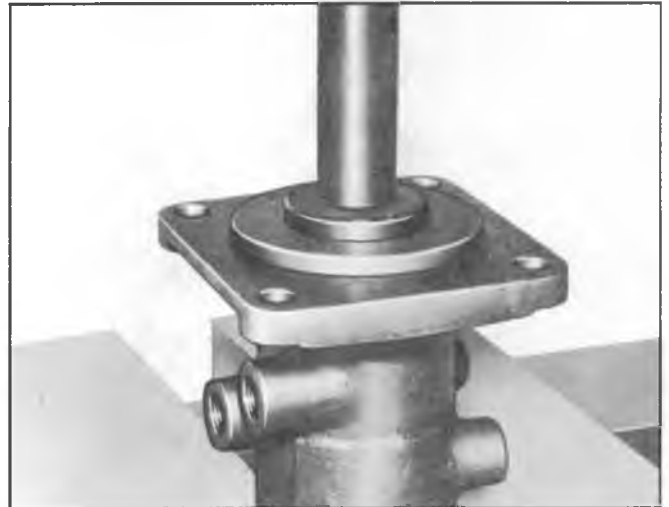
Fig. 29--Removing Top Cover Needle Bearing and Seal Using Tool J-8526-2
