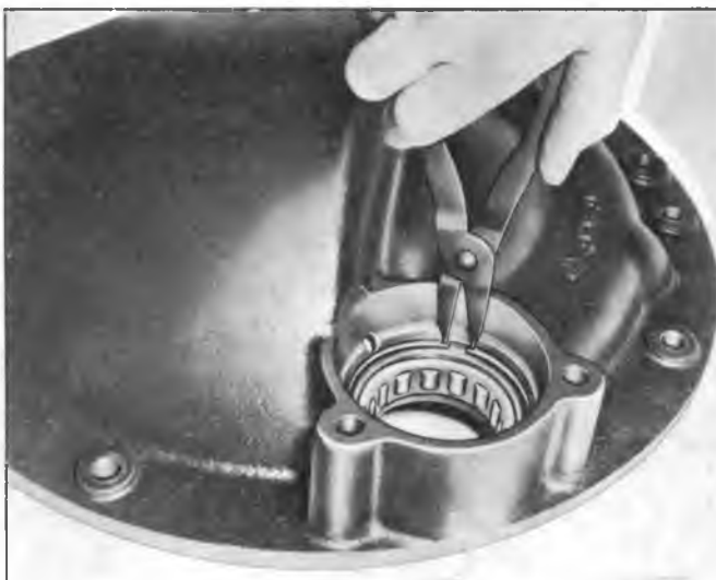
Fig. 27M--Removing Output Shaft Bearing Snap Ring
