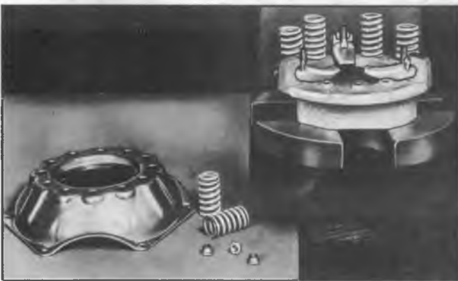
Fig. 3E--Disassembly of Clutch
