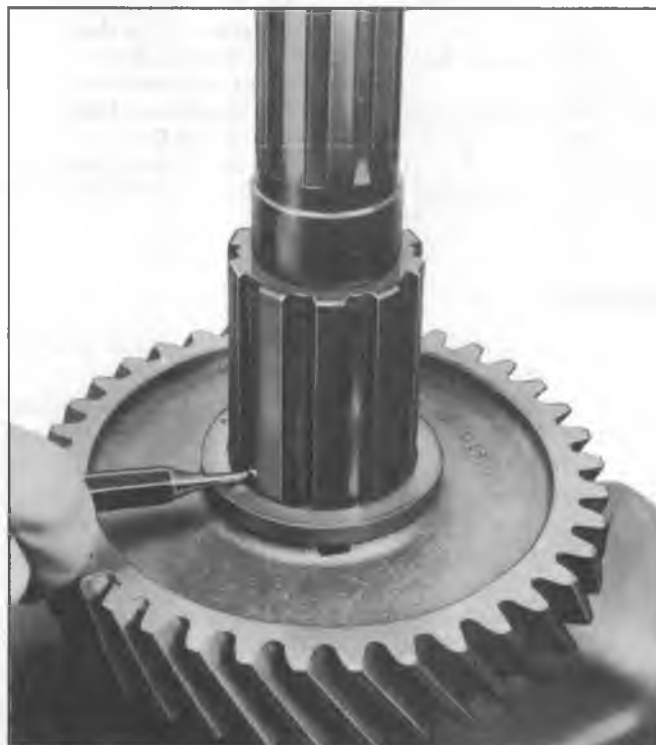
Fig. 9NP--Removing Thrust Washer and 2nd Gear
