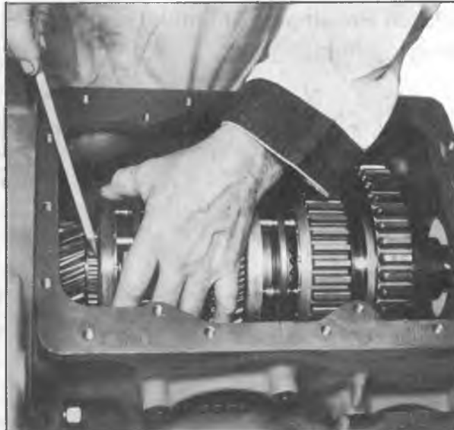
Fig. 29N--Main Drive Gear Installed
