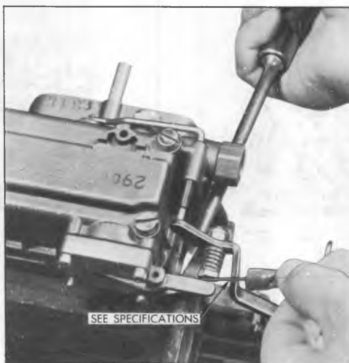
Fig. H19--Accelerator Pump Adjustment
