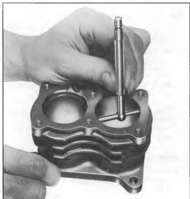
Fig. 9G—Measuring Cylinder Bore Diameter
