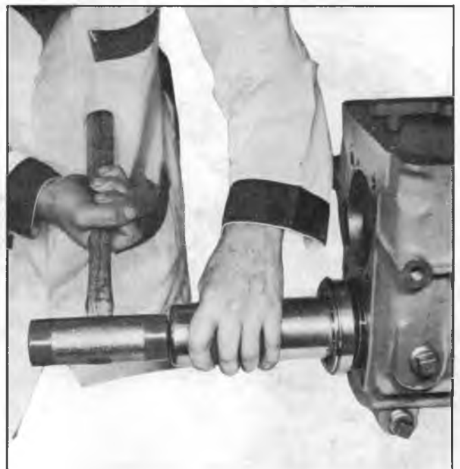
Fig. 26N--Installing Countershaft Rear Bearing
