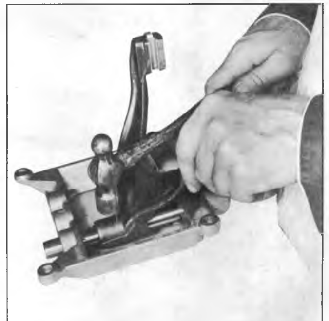
Fig. 19N--Installing 4th and 5th Shift Fork Rod Roll Pin
