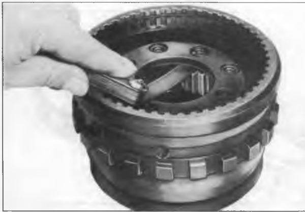
Figure 96—Checking Output Carrier Pinion End Play
