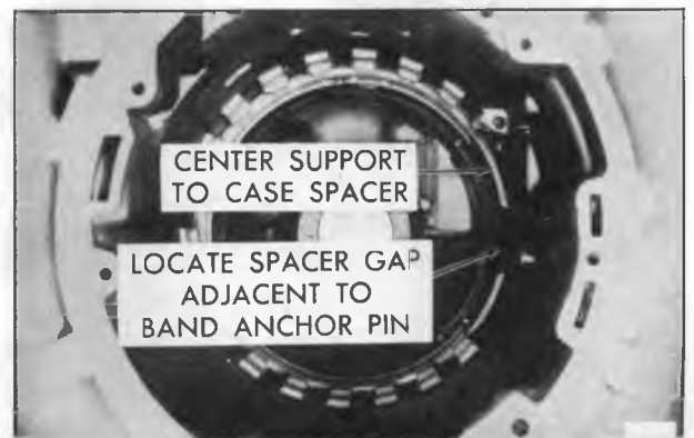
Figure 120—Positioning Center Support to Case Spacer
