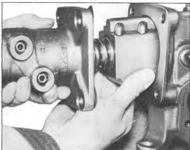
Fig. 20--Removing Top Cover, Worm, and Ball Nut Assembly
