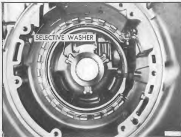
Figure 33—Removing Selective Washer
