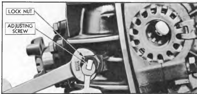
Fig. 19G--Ring Gear Thrust Pad Adjustment
