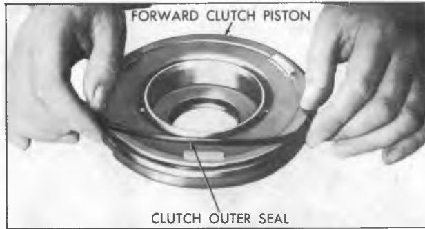
Figure 67—Removing Forward Clutch Piston Outer Seal
