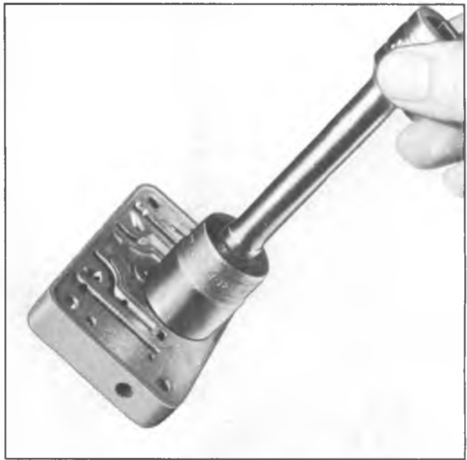
Fig. H7--Power Valve Removal
