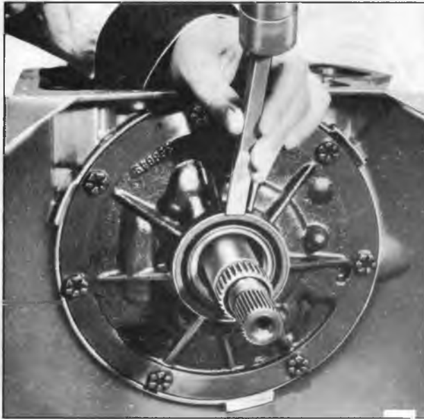
Figure 21—Removing Front Seal
