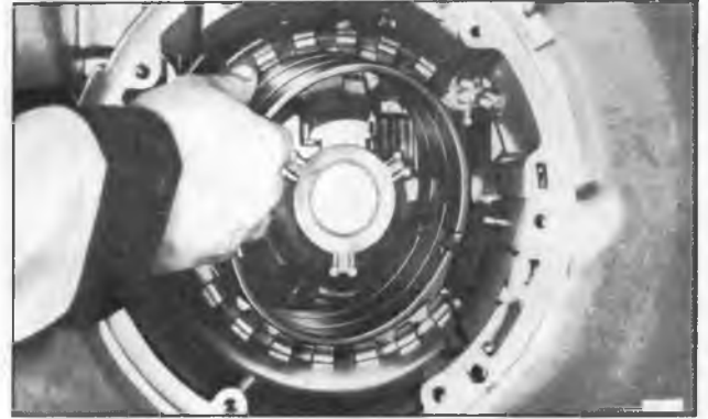
Figure 119—Installing Rear Band
