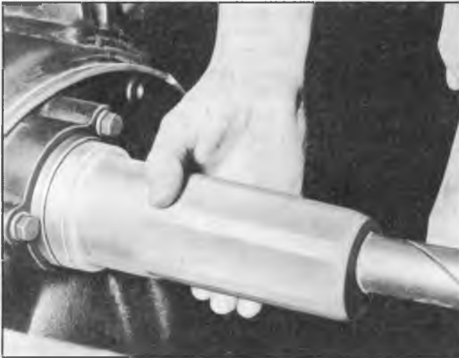
Fig. 26M--Installing Output Shaft Oil Seal Using Tool J-6419-1
