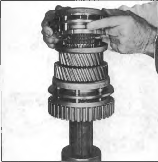
Fig. 12N--Removing 4th and 5th Synchronizer Assembly
