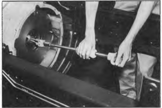
Fig. 16E--Pilot Bearing Replacement
