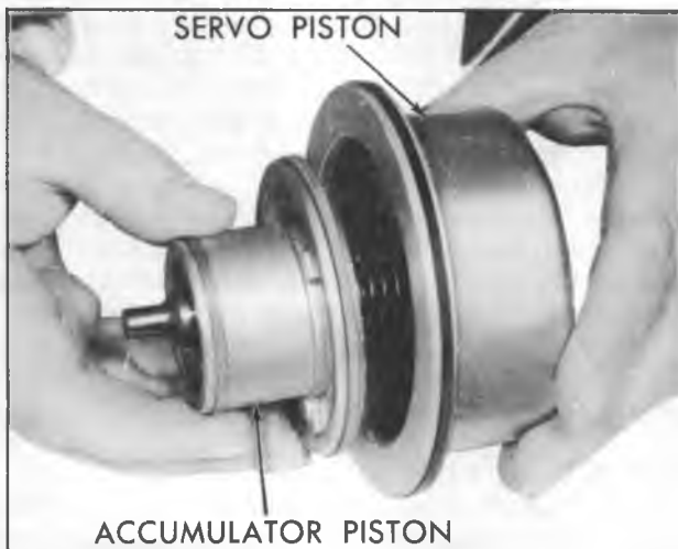
Figure 47—Removing Piston from Rear Servo Assembly
