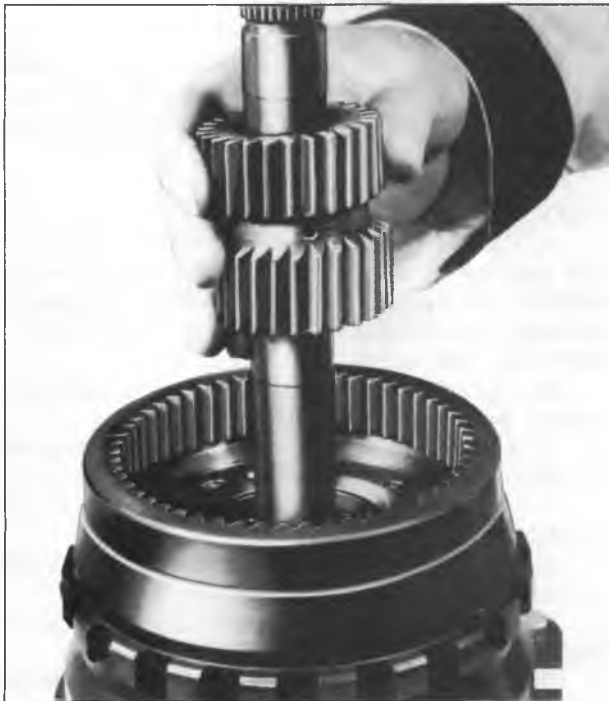
Figure 37—Removing Sun Gear
