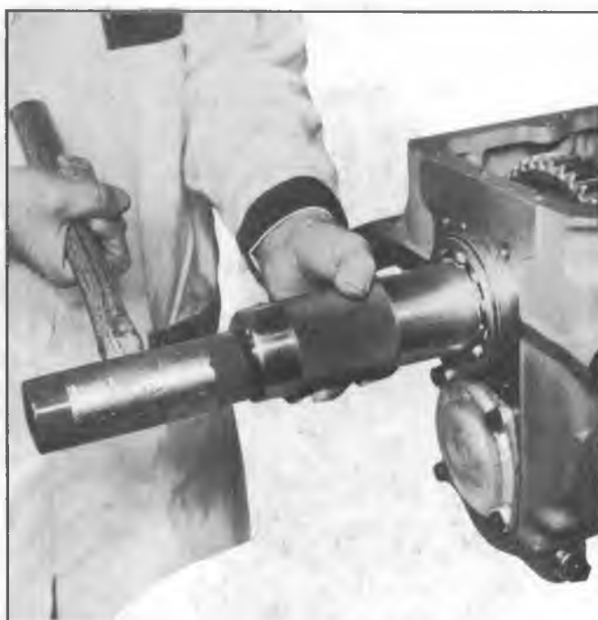
Fig. 30N--Mainshaft Rear Bearing Installation
