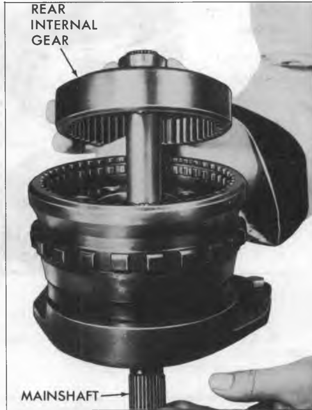
Figure 41—Removing Rear Internal Gear and Mainshaft
