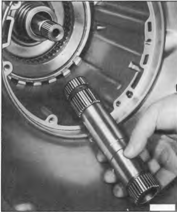
Figure 28—Removing Sun Gear Shaft
