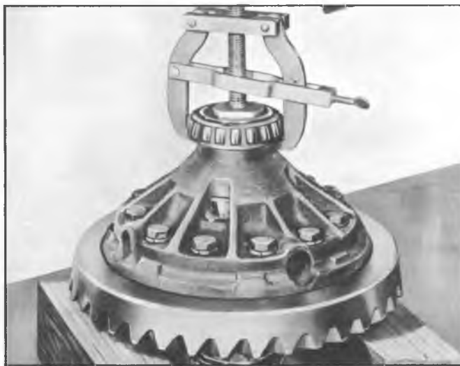
Fig. 13G--Differential Bearing Removal
