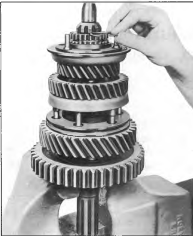
Fig. 10NP--Selecting Proper Retainer Ring
