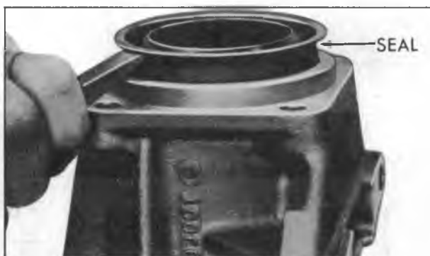
Figure 19—Removing Rear Oil Seal
