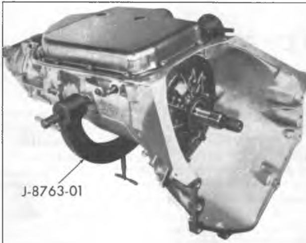
Figure 2—Transmission in Holding Fixture
