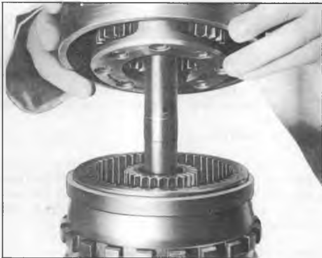
Figure 112—Installing Reaction Carrier
