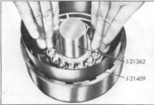
Figure 80—Installing Direct Clutch Piston
