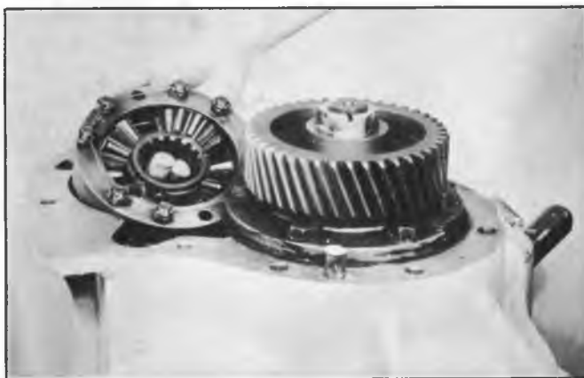
Fig. 17M--Removing Inter-Axle Differential from Carrier
