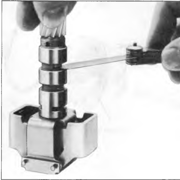
Figure 43—Checking Governor Valve Opening at Entry
