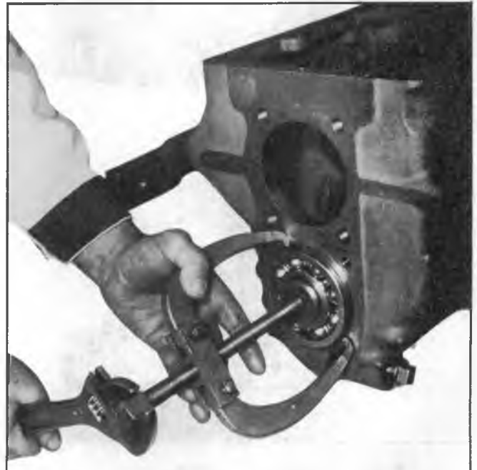
Fig. 11N--Removing Countershaft Rear Bearing
