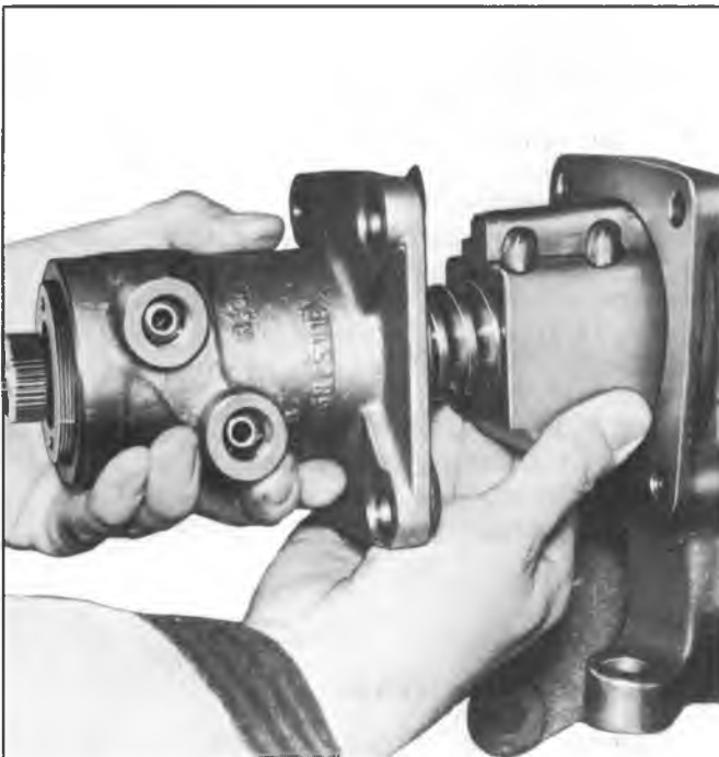
Fig. 32--Installing Top Cover, Worm and Ball Nut
