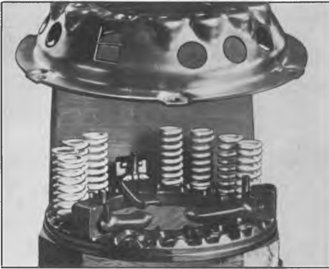
Fig. 10E--Assembling Cover and Pressure Plate
