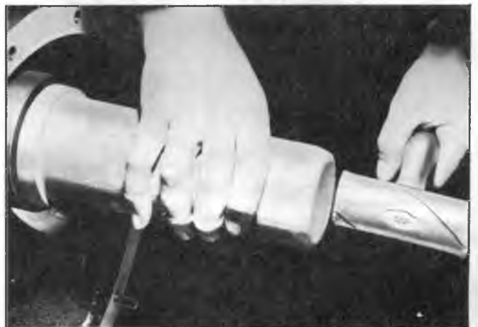
Fig. 29M--Installing Output Shaft Bearing Race With Tool J-6419-1 and -2
