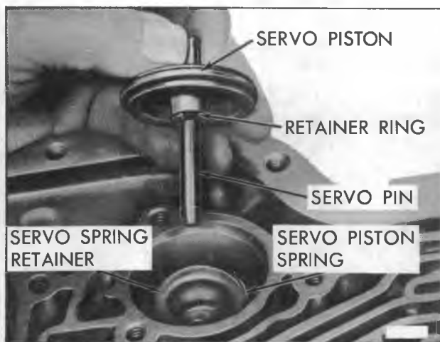
Figure 18—Removing Front Servo Piston Retainer Ring and Pin
