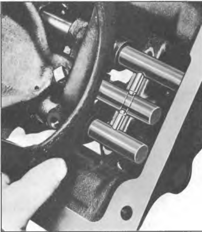
Fig. 10R--Location of Interlock Poppets
