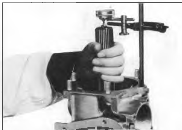
Figure 123—Checking Rear Unit End Play
