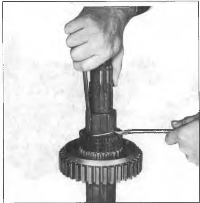
Fig. 14N--Removing 2nd and 3rd Shift Hub Sleeve Retainer Ring
