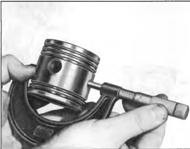
Fig. 10G—Measuring Piston Diameter
