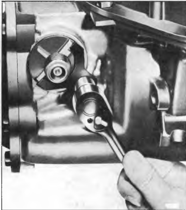
Figure 6—Removing Speedometer Driven Gear Retainer
