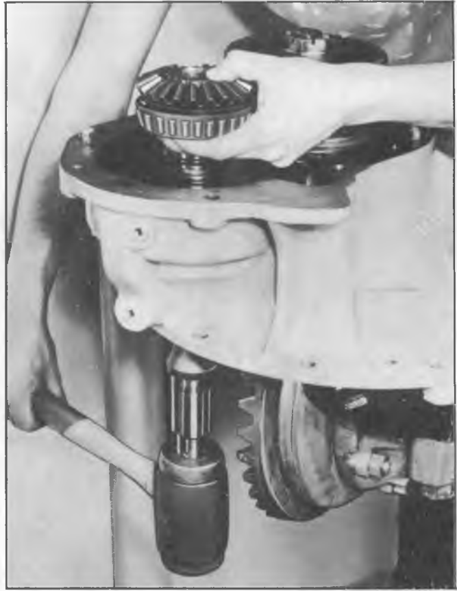
Fig. 18M—Removing Output Shaft Assembly from Carrier
