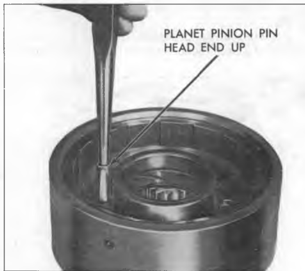
Figure 99—Installing Planet Pinion Pin
