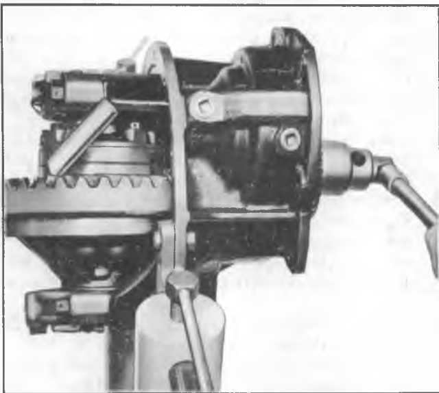
Fig. 19M—Removing Pinion Shaft Helical Gear
