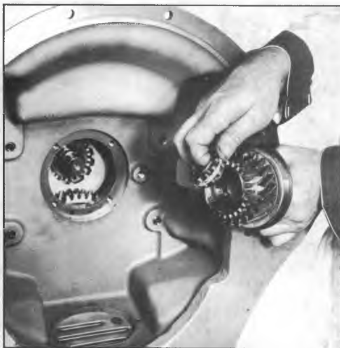
Fig. 28N--Installing Pilot Bearing
