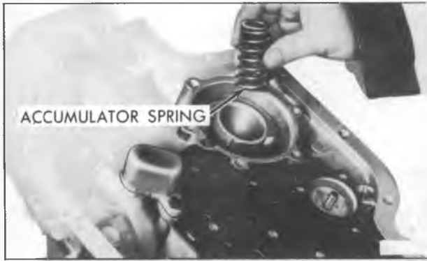
Figure 132—Installing Rear Accumulator Spring
