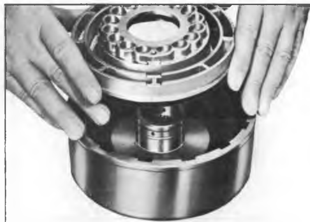
Figure 75—Removing Direct Clutch Piston Assembly
