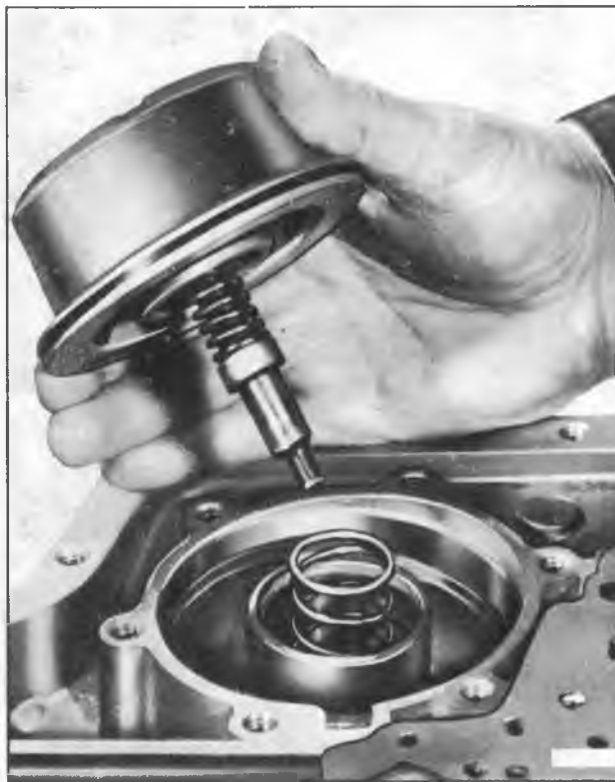
Figure 13—Removing Rear Servo Assembly
