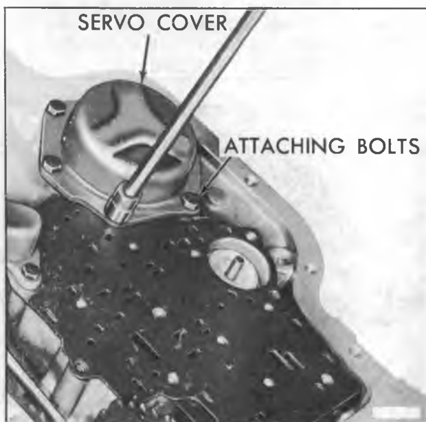
Figure 12—Removing Rear Servo Cover
