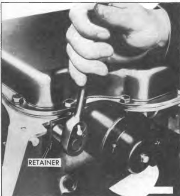
Figure 3—Removing Modulator Retainer
