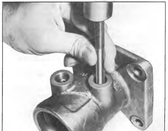
Fig. 30--Installing New Connector in Housing Using Tool J-6217
