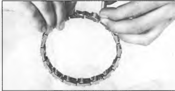
Figure 114—Installing Rollers in Clutch Cage
