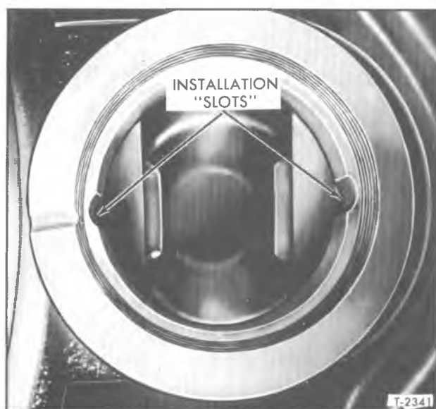
Figure 36—Wedge Cavity in Housing ("Slots" Shown)
