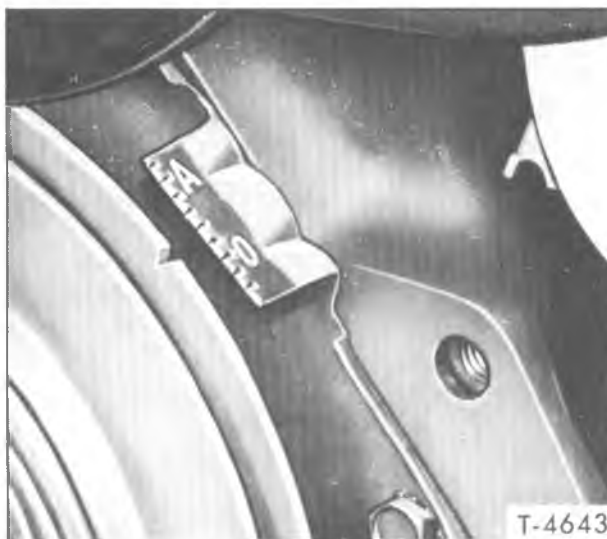
Figure 2—Timing Marks (In-Line Engine) (Typical)
