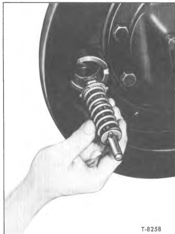
Figure 35—Installing Wedge Assembly
