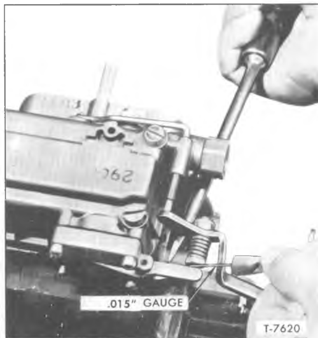
Figure 35—Accelerator Pump Adjustment
