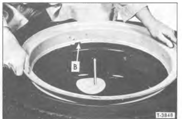
Figure 13—Position Side Ring
