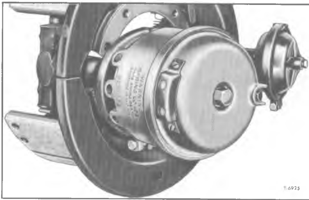
Figure 43—Brake Assembly with Super "Fail-Safe"
