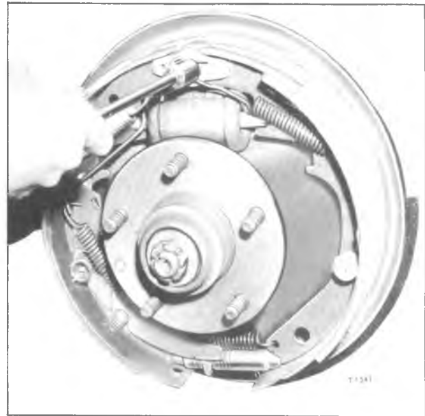
Figure 30—Unhooking Brake Shoe Return Spring
