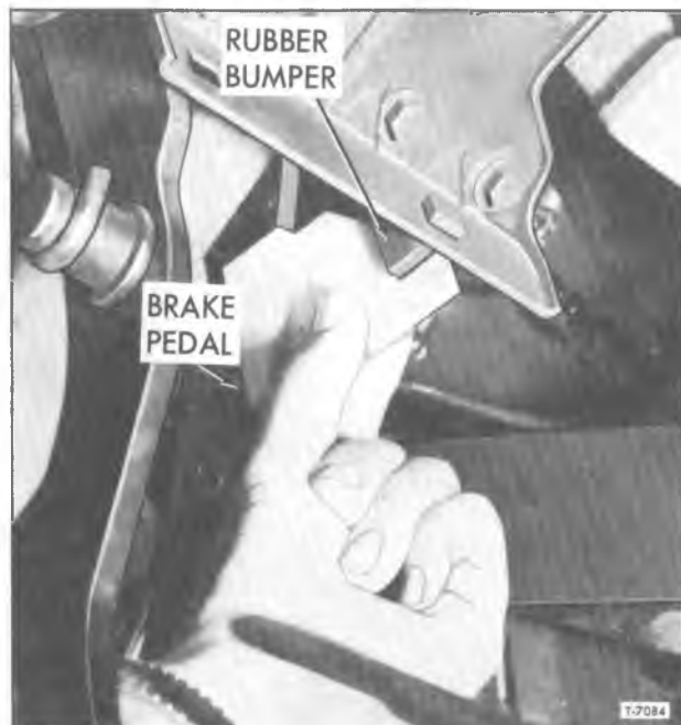
Figure 17—Pedal Travel Tool Installed
