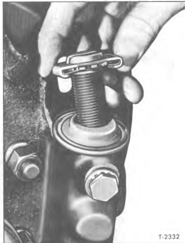
Figure 27—Installing Adjuster Bolt
