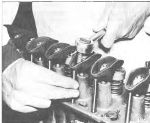
Figure 14—Valve Adjustment on In-Line Engine
