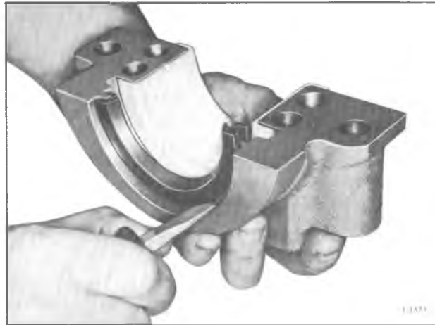
Figure 35—Removing Oil Seal from Bearing Cap
