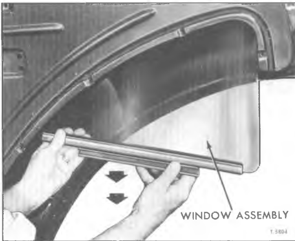
Figure 20—Removing Door Window Glass
