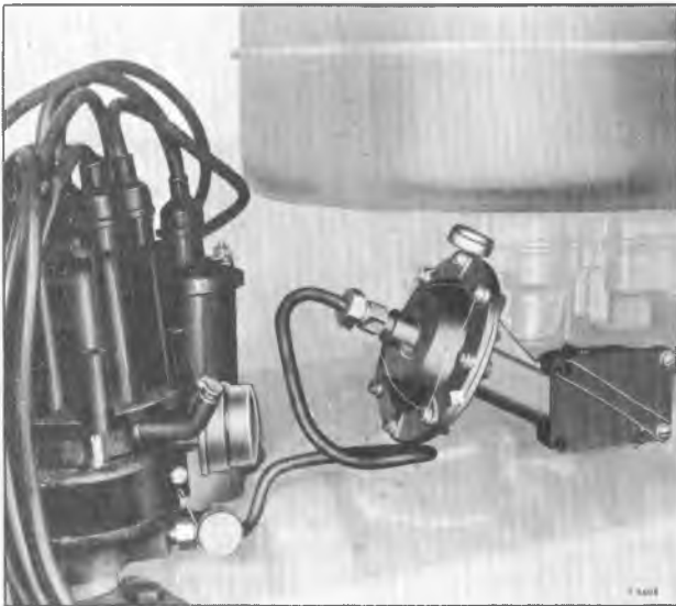
Figure 15—Distributor and Governor Mounting
