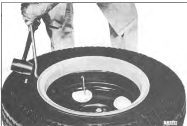
Figure 10—Loosening Tire Bead
