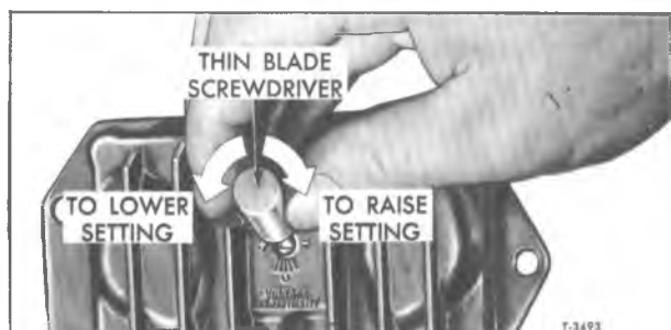
Figure 18—Adjusting Voltage Setting (Typical)
