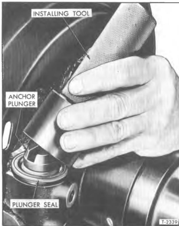
Figure 33—Installing Anchor Plunger and Seal
