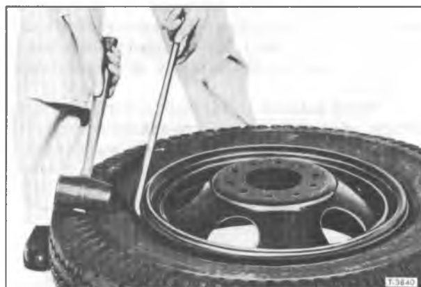
Figure 19—Starting Side Ring Removal
