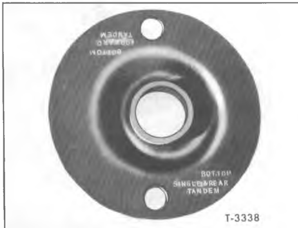
Figure 8—Electric Shift Unit Seal Markings
