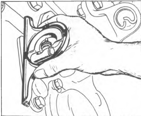
A—CHECKING ENGINE AND TRANSMISSION ANGLE
