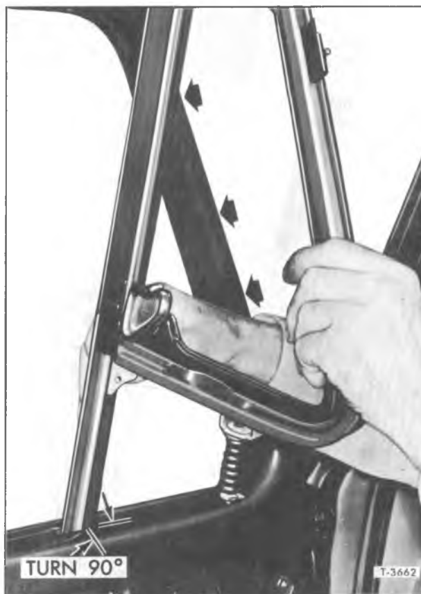
Figure 20—Vent Window Assembly Removal
