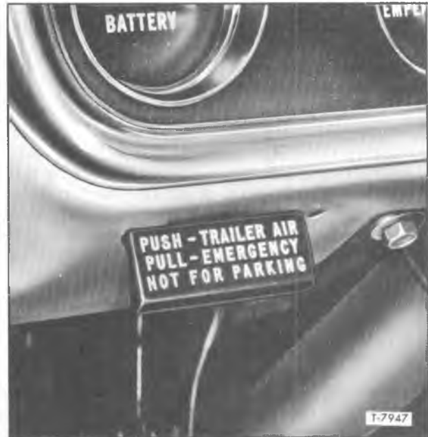
Figure 17—Emergency Control Valve Knob
