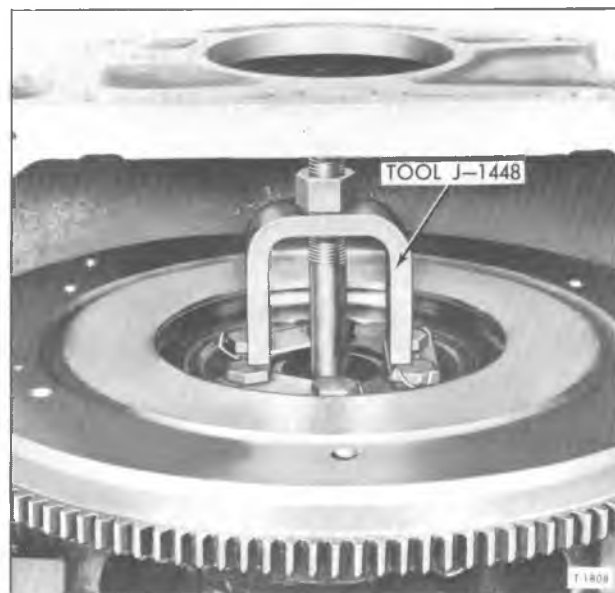
Figure 5—Pilot Bushing Removal
