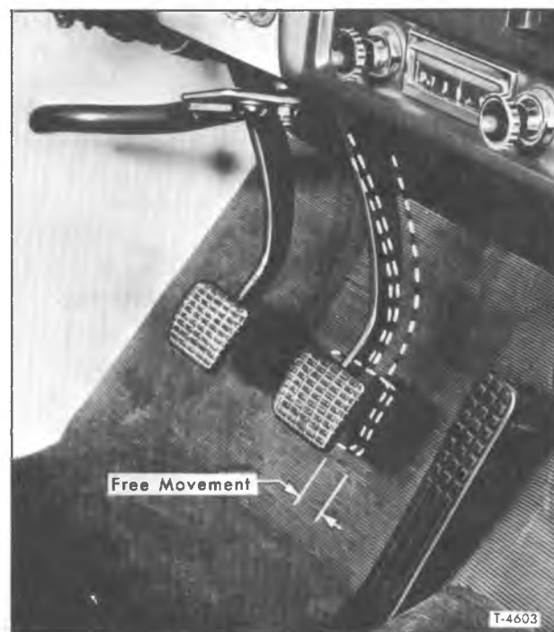
Figure 11—Brake Pedal Free Movement
