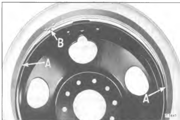
Figure 8—Slide Ring Assembly Points
