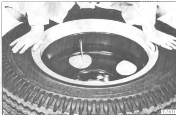
Figure 16—Checking Side Ring for Bind on Rim
