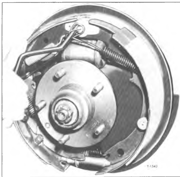
Figure 32—Installing Primary Shoe Return Spring
