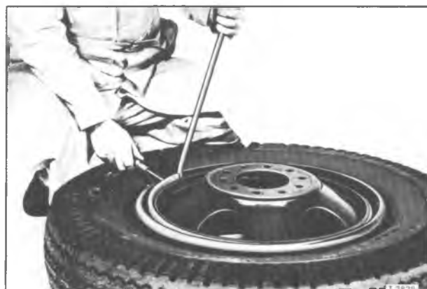
Figure 18—Raising End of Clamp Ring
