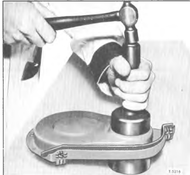
Figure 25—Installing Front Cover Oil Seal
