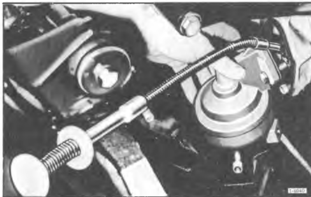
Figure 5—Installing V8 Engine Fuel Pump
