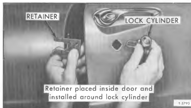
Figure 14—Door Lock Cylinder Replacement
