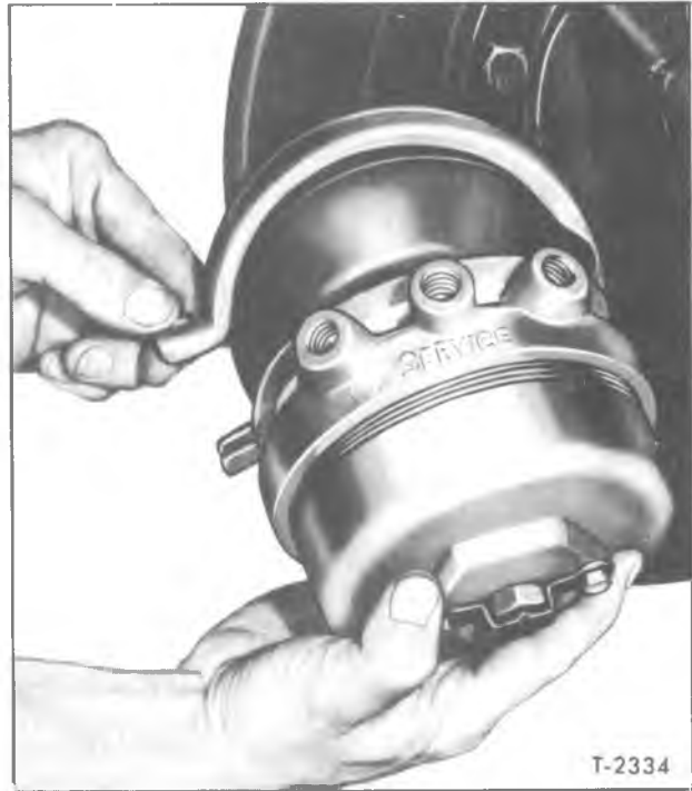
Figure 40—Removing "Fail-Safe" Assembly
