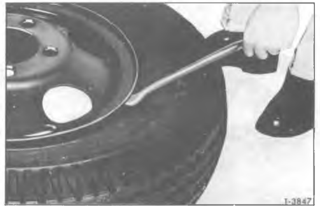
Figure 11—Loosening Tire Bead
