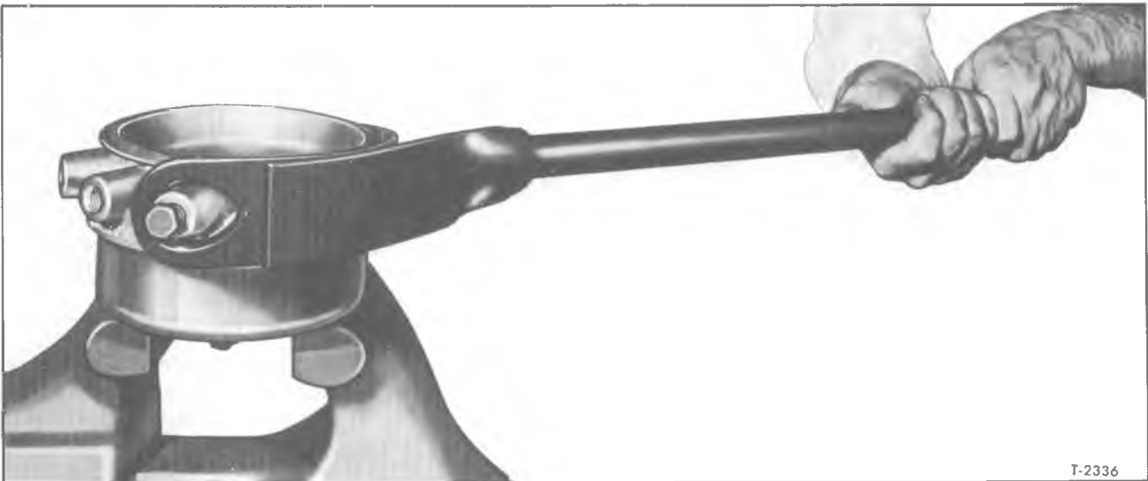
Figure 41—Removing Pressure Housing with "Strap" Wrench
