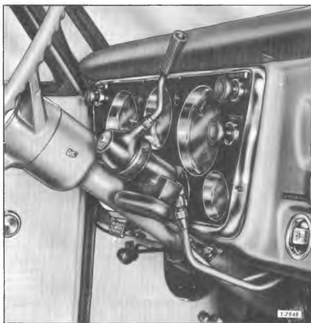
Figure 16—Trailer Brake Hand Control Valve Installed
