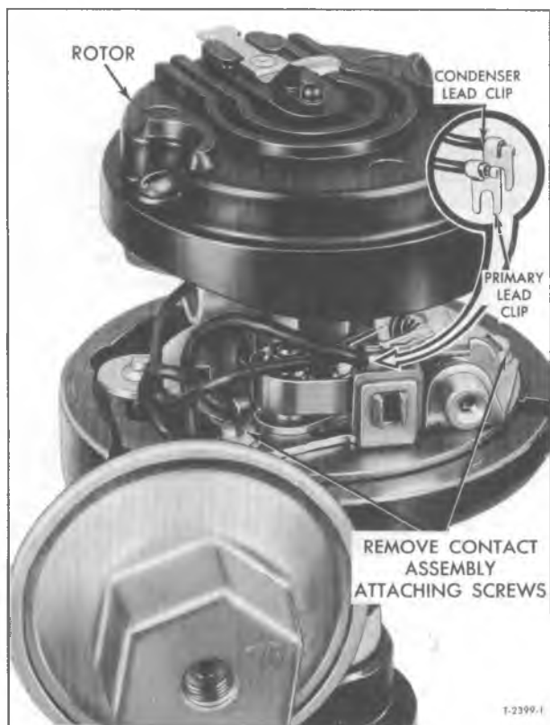
Figure 8—Distributor Contact Set Replacement
