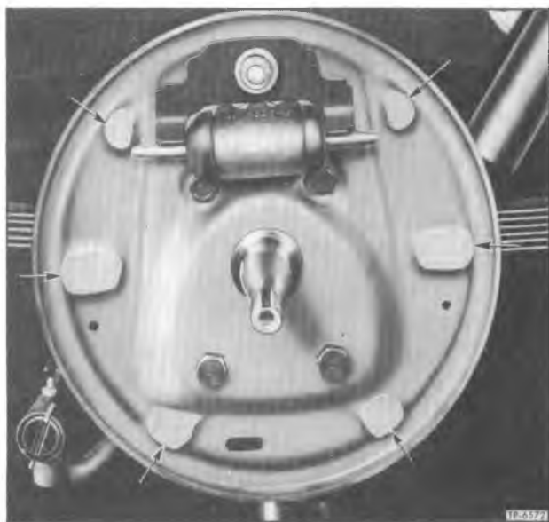
Figure 33—Brake Shoe Contact Surfaces and Backing Plate
