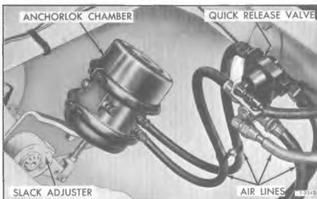
Figure 19—Anchorlok Brake Chamber Installed
