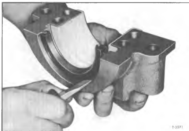
Figure 17—Removing Oil Seal from Bearing Cap
