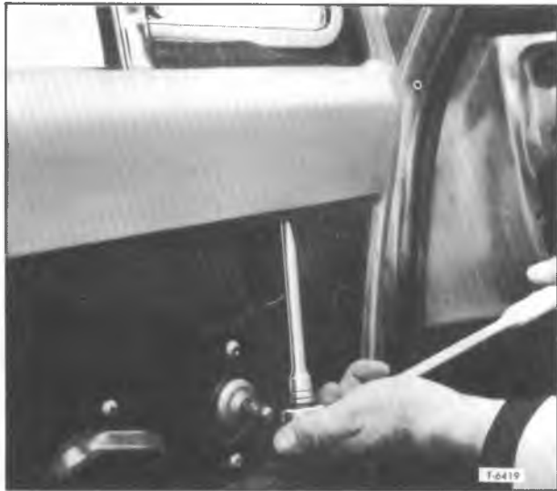
Figure 21—Adjusting Ventilator Operating Tension
