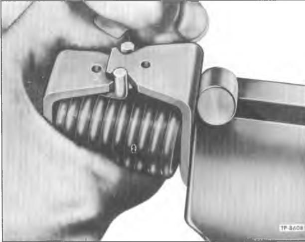
Figure 16—Disassembling Torsion Spring From Lever
