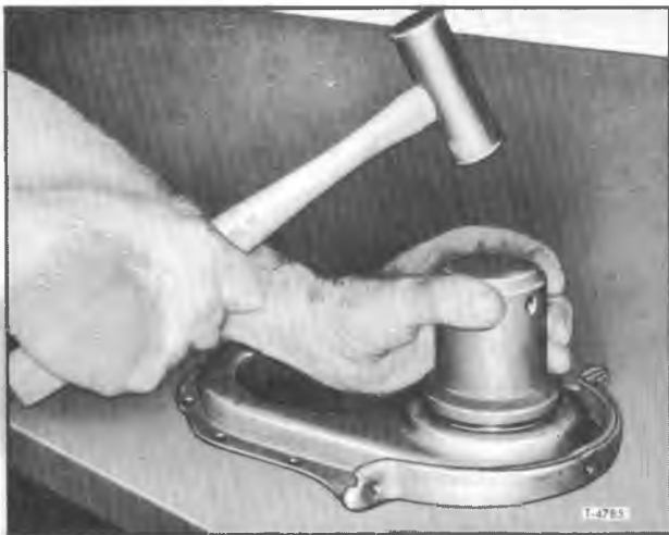
Figure 40—Installing Front Cover Oil Seal on 366 or 427 Engine (Cover Removed)
