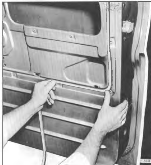
Figure 24—Installing Trim Panel Seal
