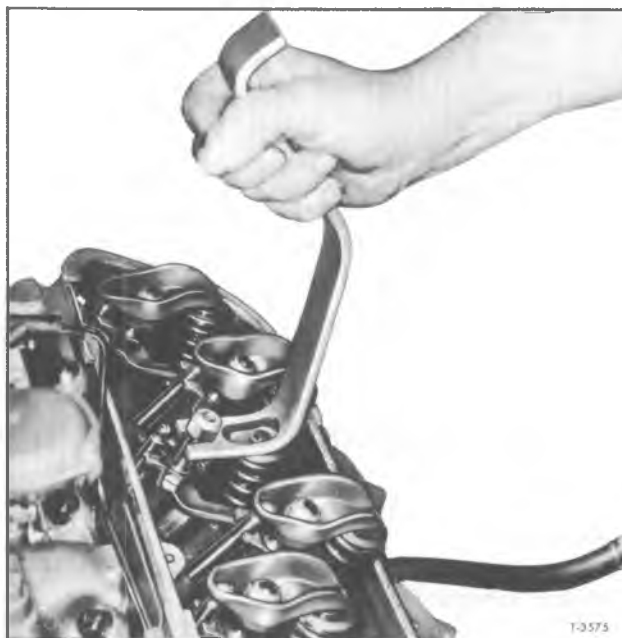
Figure 31 — Compressing Valve Spring on V8 Engine
