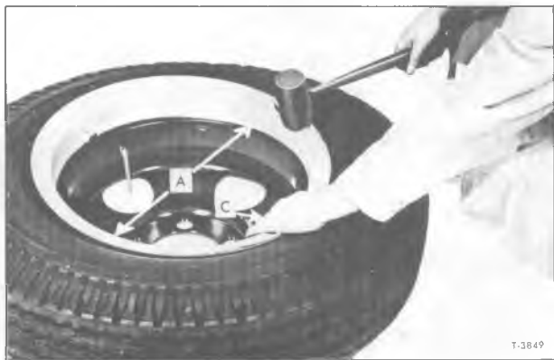
Figure 14—Positioning Ring in Rim Gutter
