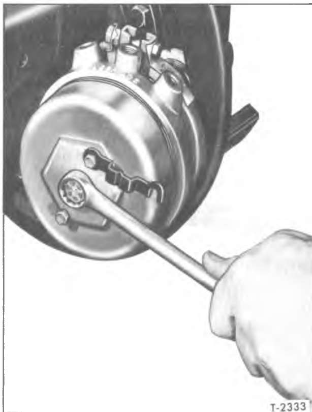
Figure 39—Compressing "Fail-Safe" Power Spring
