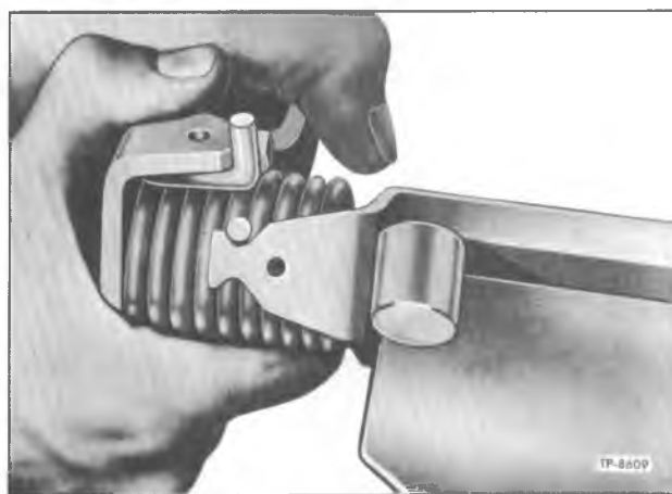
Figure 19—Assembling Torsion Spring and Levers (Eaton)
