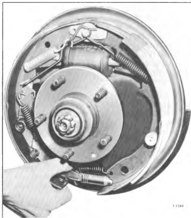
Figure 34—Checking Operation of Actuating Lever
