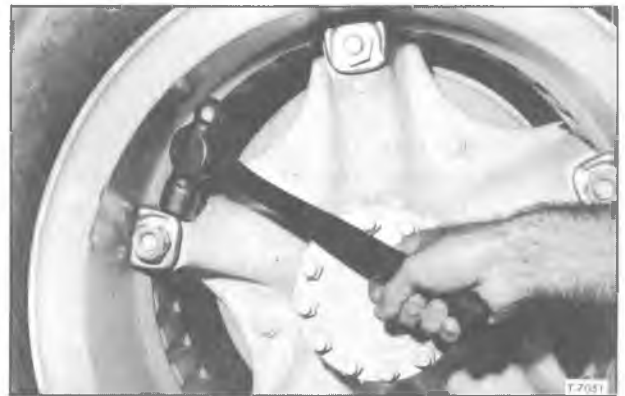
Figure 4—Clamp Removal (Dual Spoke Wheel)
